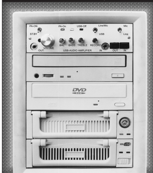
PHOTO 3: The USB audio amplifier.
