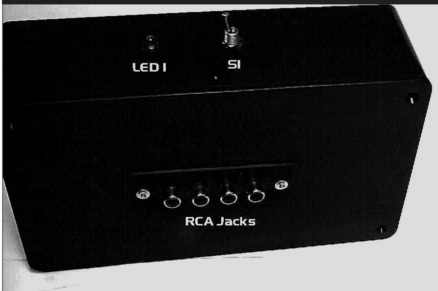
PHOTO 3: Back of device showing RCA jack input.
