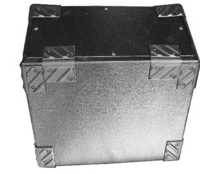
PHOTO 13: Protecting the box with plastic corners.
