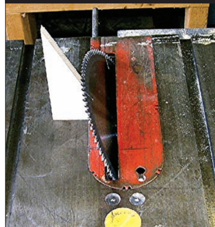
PHOTO 2: Using a cutoff to set the blade angle.
