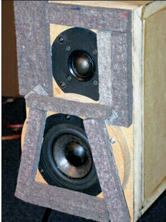
PHOTO 6: Baffle with full treatment of felt.
