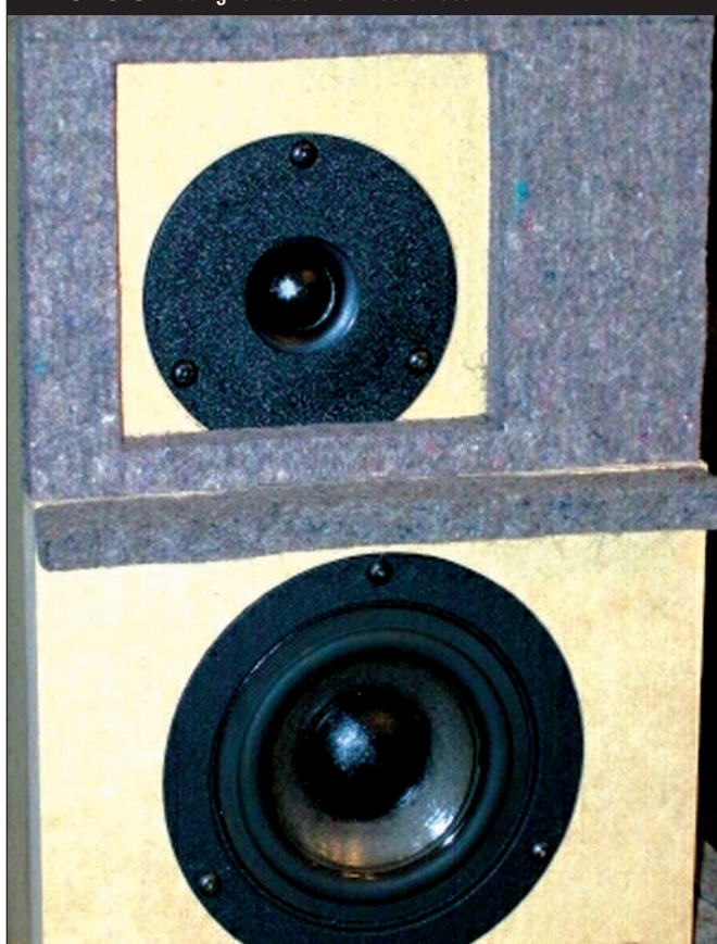
PHOTO 3: Adding felt block to tweeter face.
