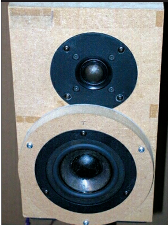
PHOTO 6: Baffle with full treatment of felt.
