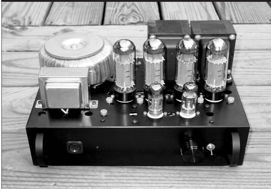
PHOTO 1: 20W per channel amplifier. Note pin jacks near each output tube, and ground pin jack near amplifier front. Bias pot shafts are visible to rear.
