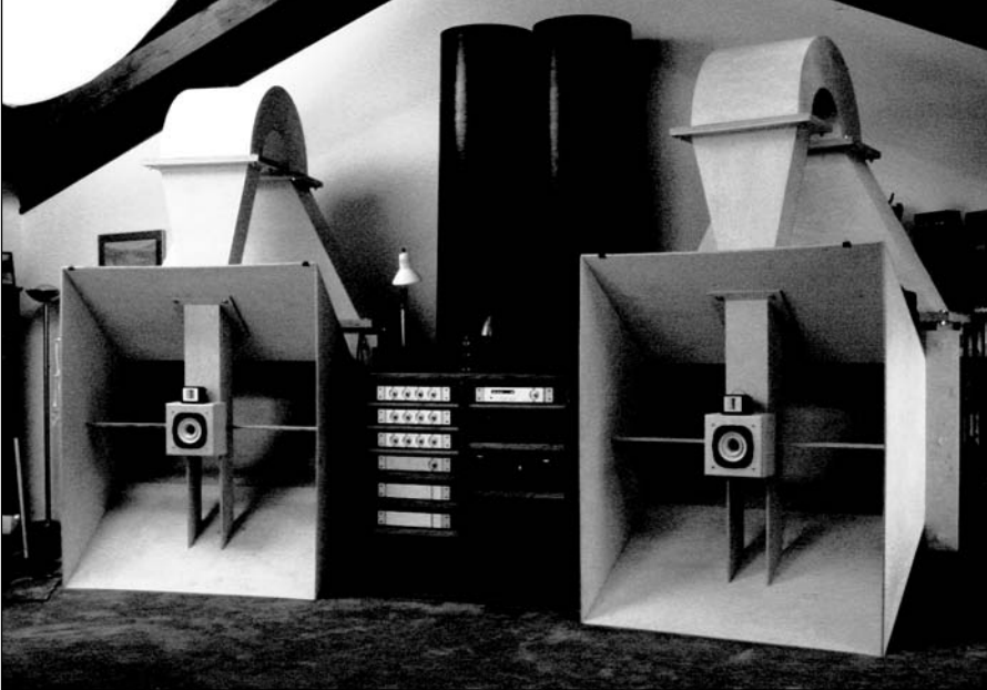
PHOTO 1: THE SYSTEM WITH THE DX4 DRIVERS AND TAD PR-R9 RIBBON TWEETERS.
