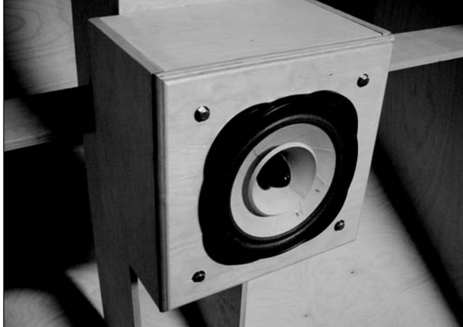
FIGURE 6: DX4 IN KLEINHORN WITH EL PIPE-O AND TAD PT-R9 RIBBON TWEETER DRIVEN BY CURRENT SOURCE AND HIGH-PASS FILTERED WITH 12DB/OCT AT 10KHZ. ALL DRIVERS IN PHASE. DOTTED LINE SHOWS TWEETER RESPONSE.
