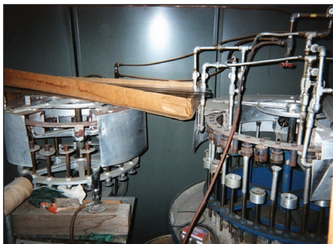
PHOTO 6: Left: used to burn in brands. Right: used for baking bases on tubes. Set up for either 217-C or 2C53 bases.
