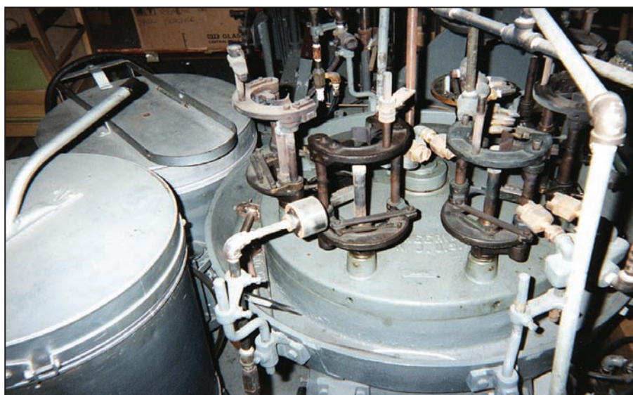
PHOTO 2: Eisler 8 head sealer (octal size bulbs). Annealing ovens to left of sealer. (Photos by Eric Barbour; captions supplied by Ronalee Elsberry).
