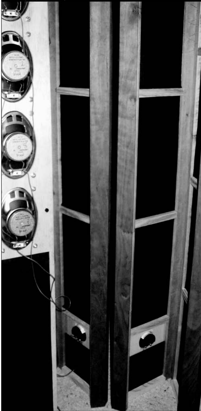
PHOTO 13: THE PANEL BRACING AND ACOUSTIC ABSORPTION MATERIAL STUCK IN PLACE.
