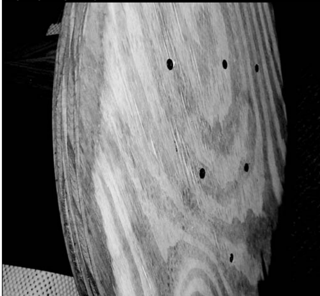
PHOTO 11: A CIRCULAR PLYWOOD PLINTH, WITH SIX SCREWS ATTACHING IT TO THE CABINET.
