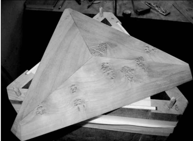
PHOTO 8: COMPLETED CAP PIECE AND THE POSITIONING DOWELS ON THE CABINET PILLARS.
