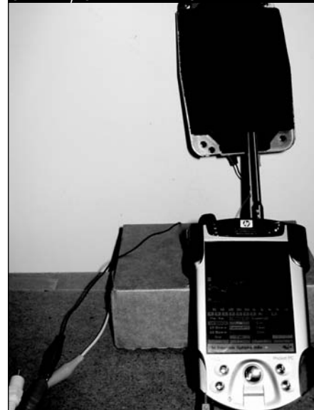
PHOTO 2: TESTING THE PINK NOISE RESPONSES OF A DRIVER USING THE IE33. THE MEASUREMENT MICROPHONE (EMERGING FROM THE IE33 JACKET AND POINTING AT THE SPEAKER) IS A TYPE II DEVICE.
