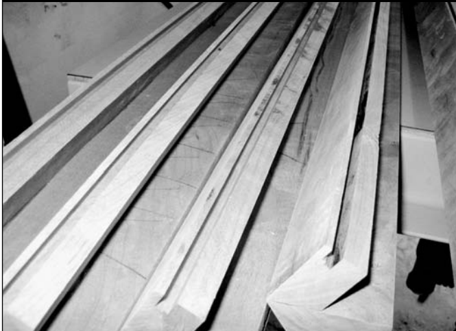
PHOTO 4: PILLAR PIECES RABBETTED FOR PLYWOOD PANELS.
