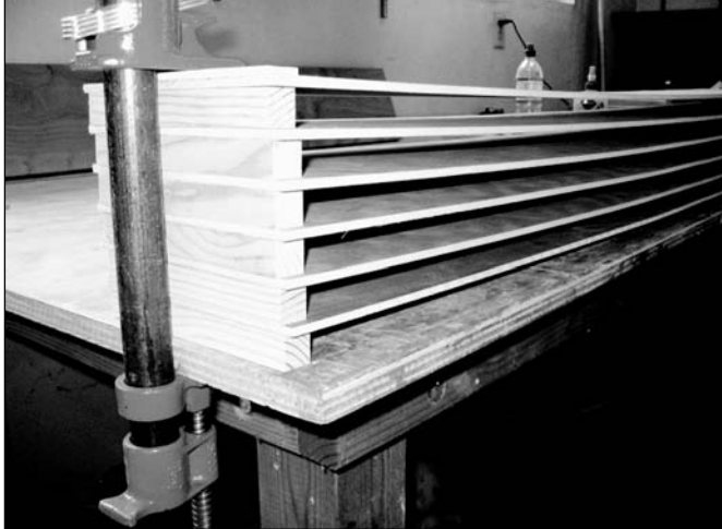
PHOTO 6: CLAMPING THE SIDE PANEL SPACERS AFTER APPLYING GLUE.
