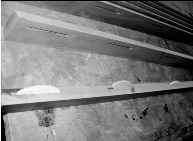
PHOTO 4: PILLAR PIECES RABBETTED FOR PLYWOOD PANELS.
