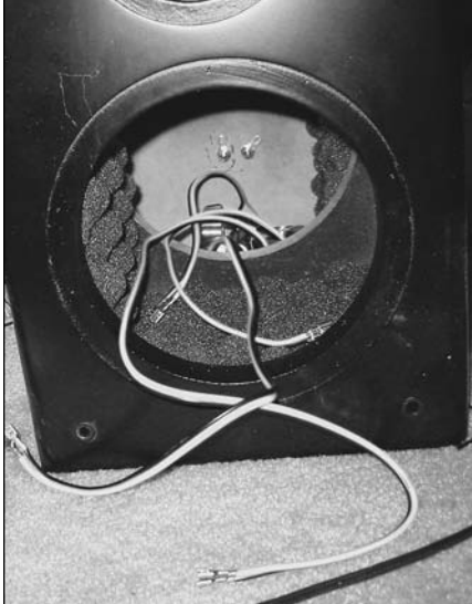
PHOTO 8: THE MANUAL ADVISES PUTTING THE CROSSOVER NEAR THE REAR. I SUGGEST IT WOULD BE EASIER TO LOCATE IT NEAR THE FRONT. THE SUPPLIED WIRE LENGTHS ALLOW THIS.
