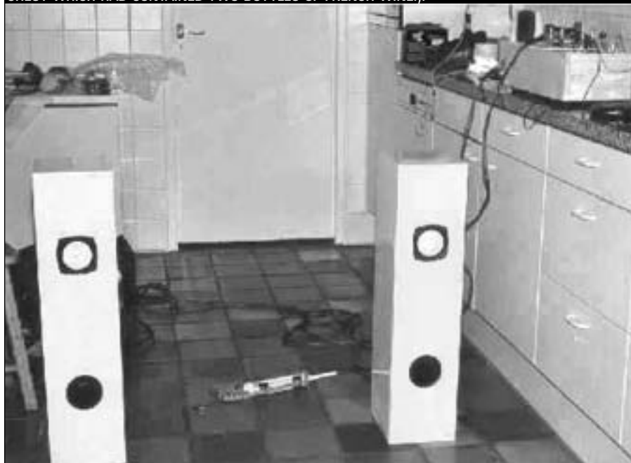
PHOTO 2: FINISHED SPEAKERS DURING AN INITIAL LISTENING TEST IN OUR KITCHEN, WITH PROTOTYPE OF THE SE TUBE AMP ON THE DRAINING BOARD (QUITE APPROPRIATELY BUILT INTO A CHEST WHICH HAD CONTAINED TWO BOTTLES OF FRENCH WINE!).
