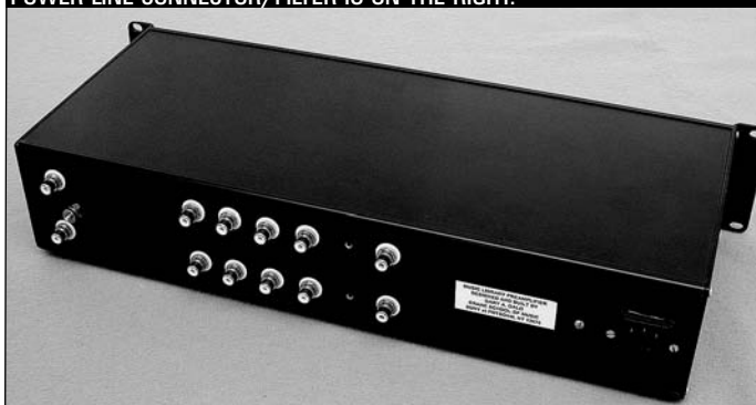
PHOTO 7: REAR PANEL OF THE ASSEMBLED PREAMP. I INSTALLED ONLY FOUR LINE INPUTS, BUT YOU COULD EASILY ADD A FIFTH. THE FUSED IEC POWER LINE CONNECTOR/FILTER IS ON THE RIGHT.
