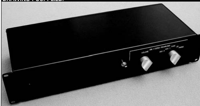
PHOTO 6: FRONT VIEW OF THE ASSEMBLED MUSIC LIBRARY PREAMP IN THE SESCOM 2RU7 RACK CHASSIS. THE PLASTIC FRONT PANEL LABEL WAS MADE BY A LOCAL HOBBY SHOP FROM A CAD DRAWING I SUPPLIED.
