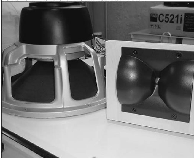
PHOTO 11: FRONT VIEW OF 2404H TWEETER ASSEMBLY NEXT TO 15" UNIVERSITY C15W LOW-FREQUENCY DRIVER.
