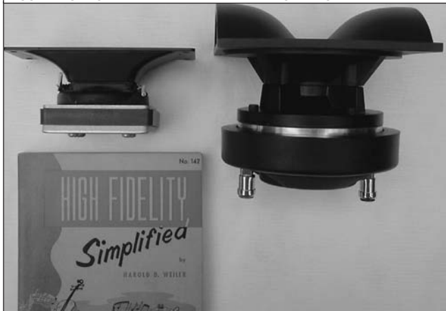
PHOTO 2: THE DIFFERENCES BETWEEN THE JBL 2404H AND THE EV T35 HORNS (VIEW IS FORWARD LOOKING AFT).
