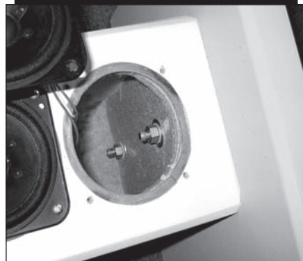
PHOTO 5: Lowest driver cutout showing bolts.
