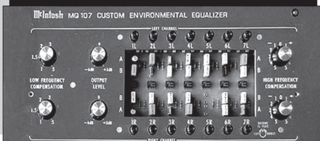
PHOTO 7: The McIntosh MQ107 equalizer, with cover removed.
