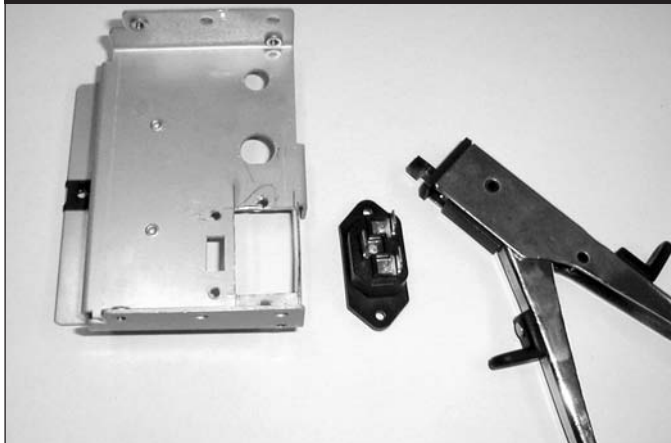
PHOTO 14: ENLARGING THE CUTOUT FOR IEC RECEPTACLE.
