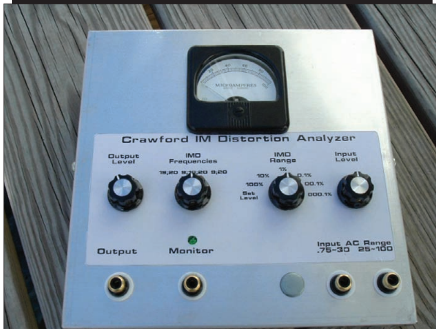
PHOTO 1: Homemade distortion analyzer.
