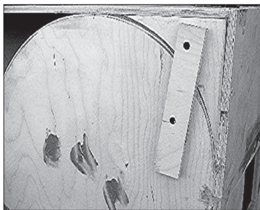
PHOTO 18: Using a caul to align filler.
