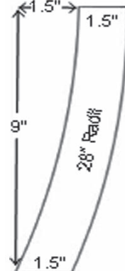
FIGURE 13: Rear horn brace.
