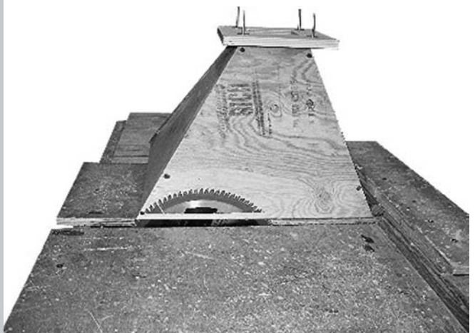
PHOTO 10: Trimming the horn mouth with a panel cutting jig.
