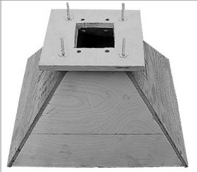
PHOTO 10: Trimming the horn mouth with a panel cutting jig.
