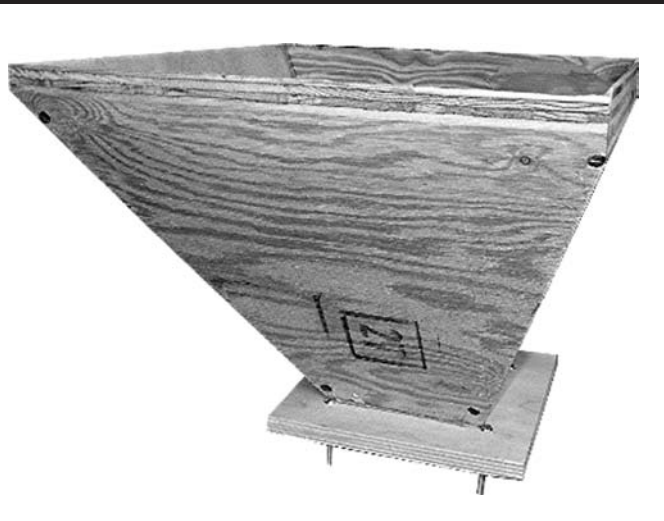
PHOTO 12: The trimmed horn ready for installation.
