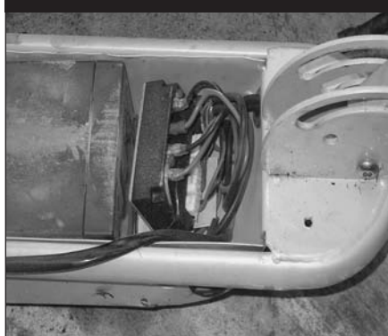
PHOTO 4: DC speed controller from scooter.
