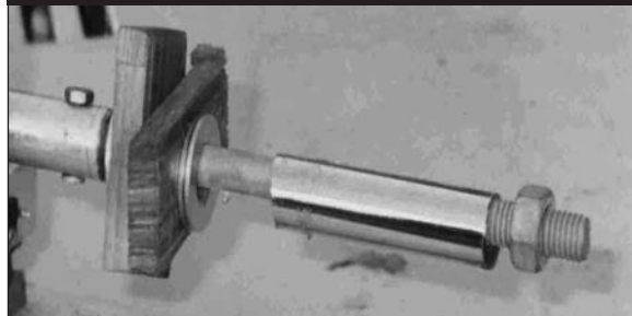
PHOTO 6: Close-up of the motor shaft and adapter.
