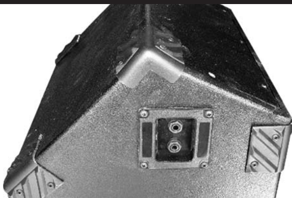
PHOTO 14: Dual phone jacks for daisy-chaining.
