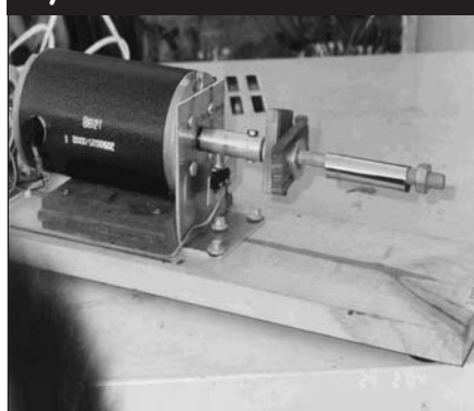
PHOTO 5: Complete motor assembly of winder.
