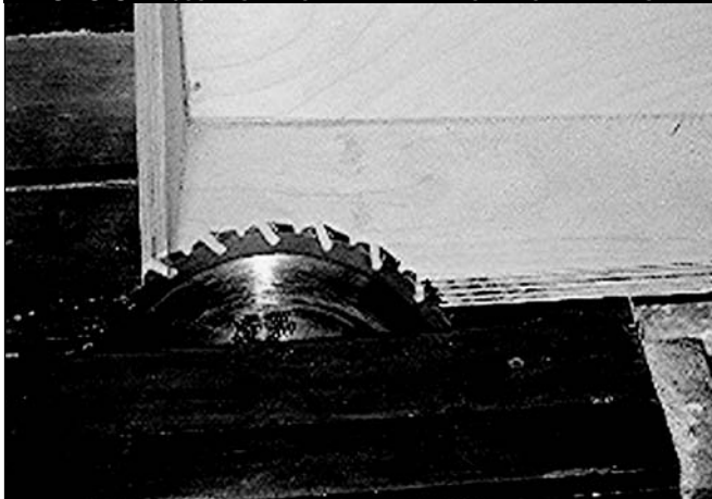
PHOTO 3: ADJUSTING THE SAW BLADE TILT TO THE CABINET ANGLE.
