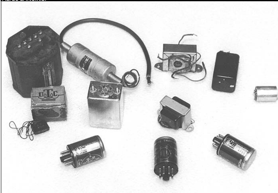
PHOTO 2: A VARIETY OF INPUT TRANSFORMERS BY UTC, HAMMOND, ELECTRA-PRINT, AND ALTEC-LANSING.
