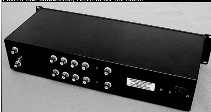
PHOTO 7: REAR PANEL OF THE ASSEMBLED PREAMP. I INSTALLED ONLY FOUR LINE INPUTS, BUT YOU COULD EASILY ADD A FIFTH. THE FUSED IEC POWER LINE CONNECTOR/FILTER IS ON THE RIGHT.
