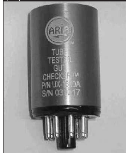
PHOTO 3: HOUSING ASSEMBLY FOR 1,500\mu\text{S} TRANSCONDUCTANCE STANDARD.
