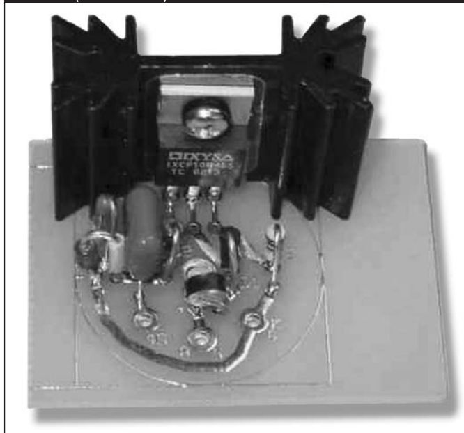
PHOTO 2: FINALIZED PROTOTYPE CIRCUIT BOARD WITH LARGE HEATSINK (FOR TESTING).
