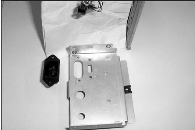
PHOTO 14: ENLARGING THE CUTOUT FOR IEC RECEPTACLE.
