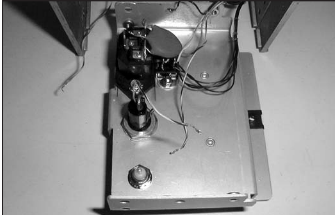
PHOTO 16: 3-LEAD CAPACITOR INSTALLATION.
