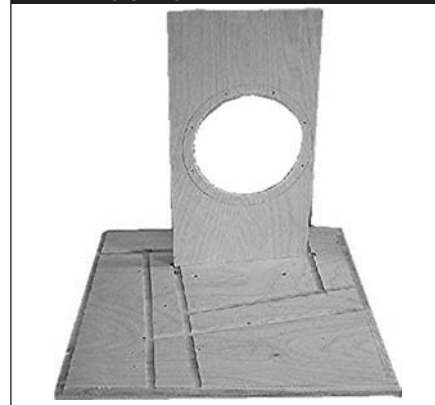
PHOTO 4: ATTACHING PLATE A TO ONE SIDE.
