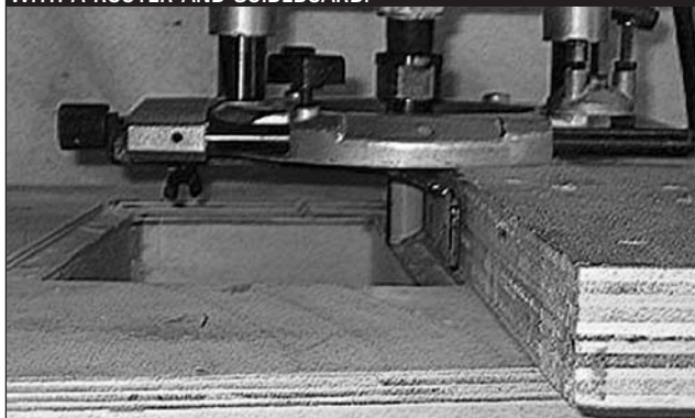
PHOTO 12: FLANGING A PORTHOLE WITH A ROUTER AND GUIDEBOARD.
