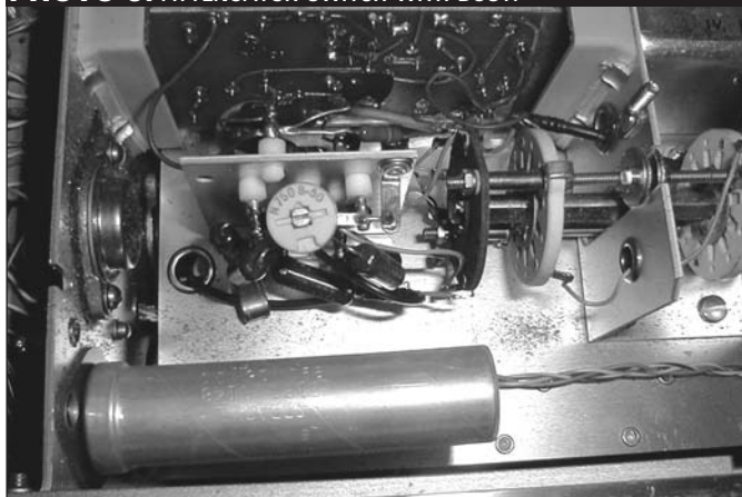
PHOTO 5: ATTENUATOR SWITCH WITH DUST.
