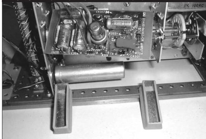
PHOTO 7: BOARD SLIDES WITH TAPE RESIDUE.
