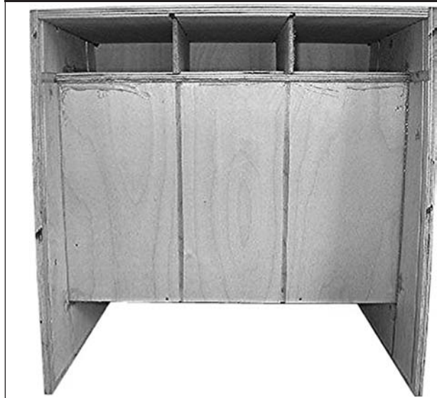
PHOTO 7: BRACES IN PLACE; NOTE RABBETS CUT INTO THE EXPOSED PLATE.
