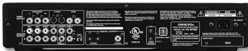
PHOTO 2: Rear panel of the DV-SP800. The player has 14 analog output channels, and both S/PDIF coax and Toslink optical digital outputs. On the video end, the player outputs component video, S-video, and standard NTSC composite.
