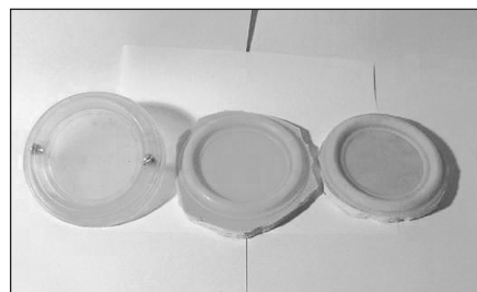
PHOTO 12: Table Top Epoxy-wood glue molds.
