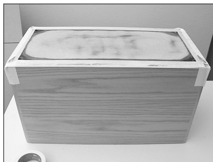
PHOTO 5: Masked and sanded, ready for attaching front panel build-up.
