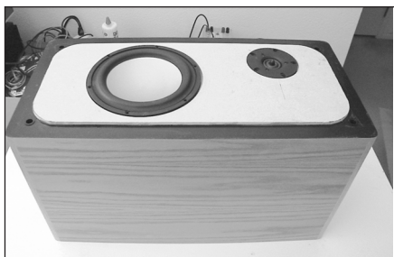
PHOTO 7: Checking driver fit after cutting holes.
