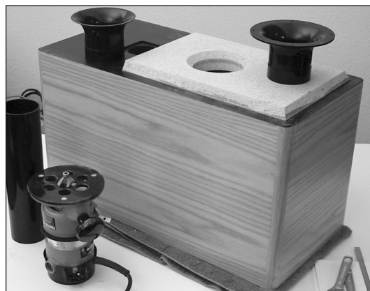
PHOTO 13: Back panel after routing for port mounting flare.
