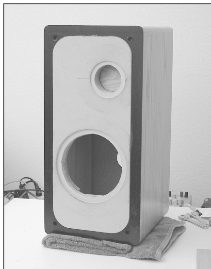
PHOTO 11: Front panel braces routed and tweeter sub-baffle installed.
