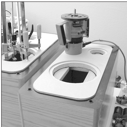
PHOTO 10: Ready to mill out woofer opening in front panel braces.
