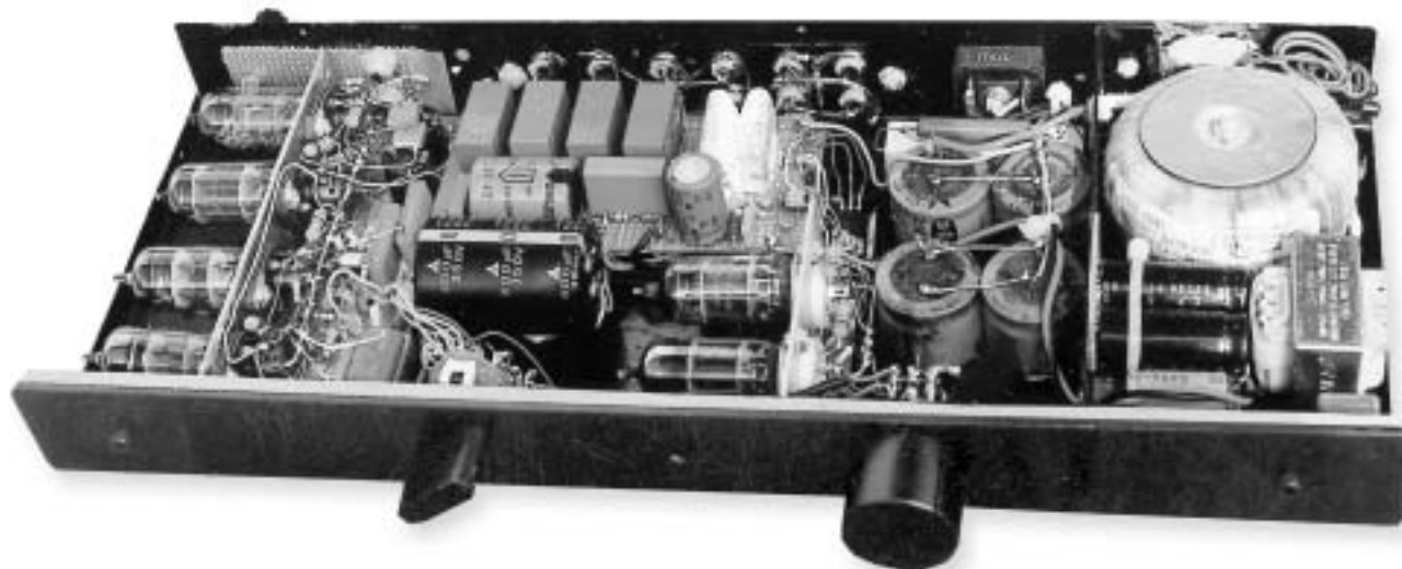
PHOTO 4: A previous project—phono and line stage preamp, based on the well-known RCA tube manual phono stage with the simple triode stages replaced with SRPP topology. None of my designs use negative feedback. This unit has relay input switching, a slow turn-on DC filament supply and high voltage filtering using a choke and large capacitor. The power transformer is a toroid type to which I added a high voltage winding. (There is a simple technique to accomplish this without too much difficulty.) Tubes used are 12AX7, 12AT7 and 12AU7. All this fits neatly in a small chassis 6 \times 15 \times 1\frac{1}{2} ". I'm extremely pleased with this project as well.
