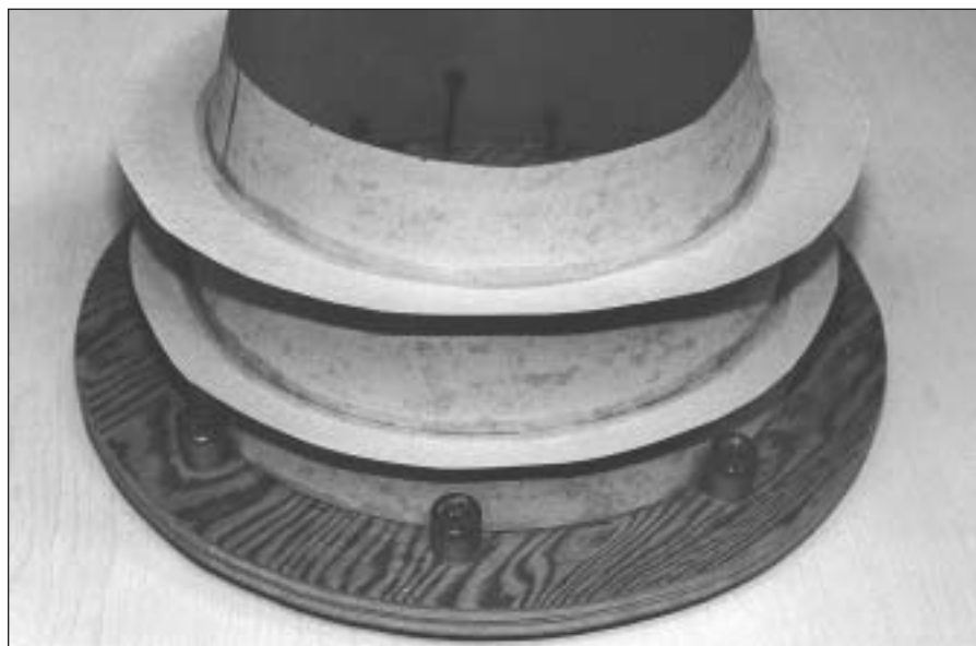
PHOTO 5: Fitting the base retainer mold sections, reinforced by a second ring.
