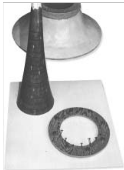
PHOTO 2: Horn extension inner mold and connecting plate.
