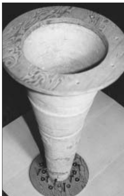
PHOTO 11: Aligning the wooden and concrete throats.
