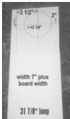
PHOTO 1: All sides of this project are the same. Since the material is \frac{3}{4} " thick, the side boards are just over 7 \frac{3}{4} ". The driver needs an opening of radius 2 \frac{1}{4} ".
