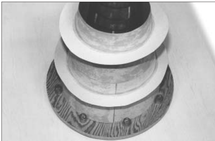
PHOTO 7: Assembling the horn mold pieces ready for casting, a dry run.
