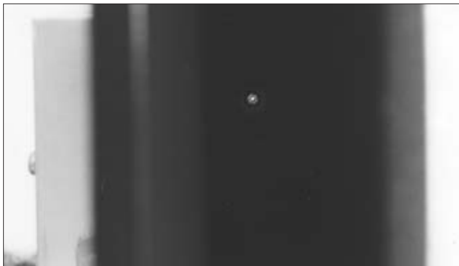
PHOTO 6: A normal plasma pattern. Note the even circular glow with a brighter point in the center. The crosshatch distortion is due to the mesh screen located just in front of the cell in the throat of the horn.
