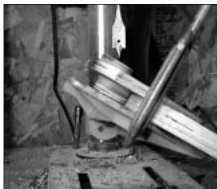
PHOTO 25: Drilling a mike stand socket.
