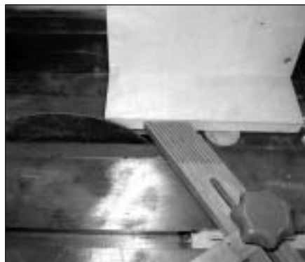
PHOTO 11: Jig and finger-board for cutting PVC lengthwise. Note abrasive table saw blade.
