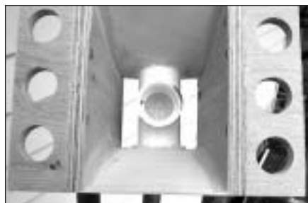
PHOTO 10: PVC "T" glued into the horn throat.
