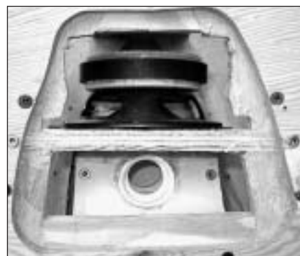
PHOTO 28: Woofer in place. Note trimming of porthole flanges to allow woofer passage.
