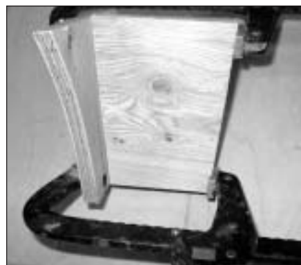
PHOTO 5: Beginning the throat horn assembly.
