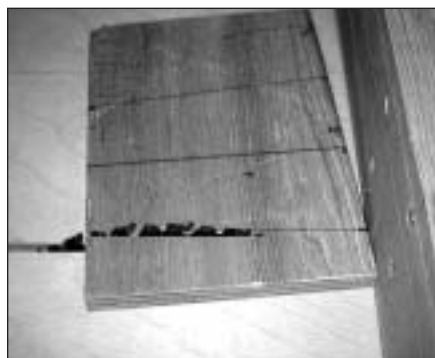
PHOTO 4: Cutting the throat horn jig.
