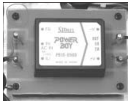
PHOTO 5: 5V power supply.
