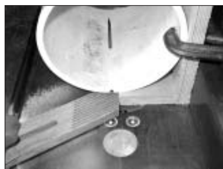
PHOTO 12: Slicing PVC. Note blade does not penetrate fully at the ends of the cut.
