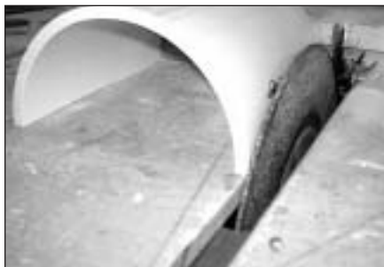
PHOTO 22: Chamfering PVC edge with the paneling jig and abrasive blade.
