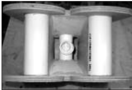
PHOTO 21: The PVC reflectors in place.
