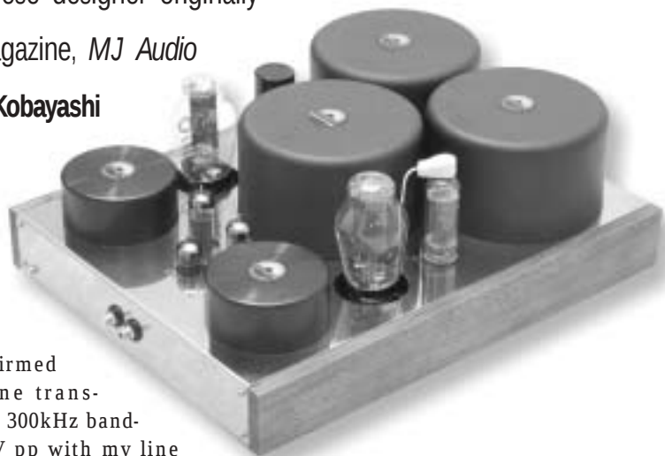
PHOTO 1: Completed SV300B- based amp.
