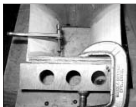
PHOTO 7: Attaching throat horn supports. Note right angle ratchet driver.
