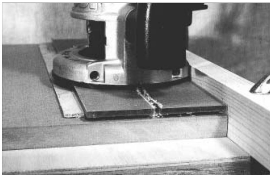
PHOTO 7: It almost makes itself. Just cut the plastic against any improvised fence.
