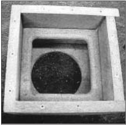
PHOTO 8: Rear view for boxes #5 and #6 showing front panel relieving.
