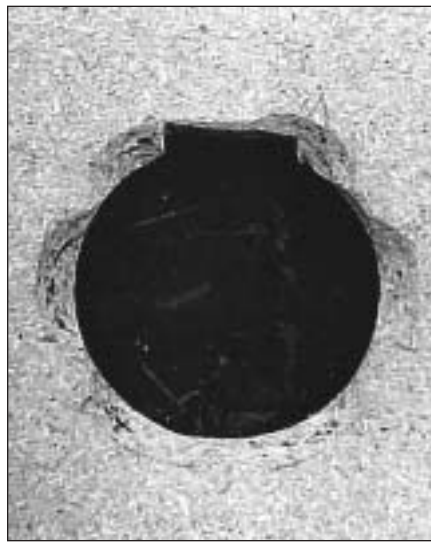
PHOTO 13: Relieving of front panel rear for W3-871s driver.
