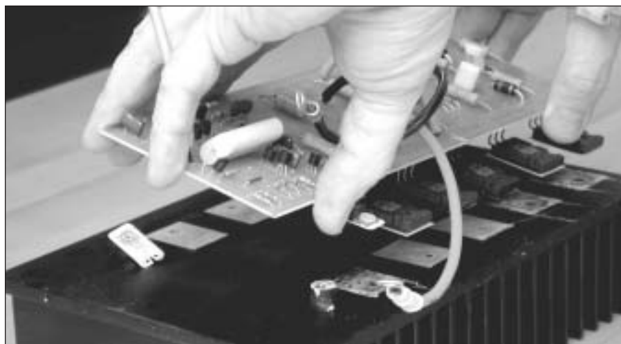
PHOTO 3: Removing the original PC board.
