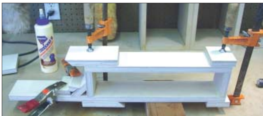
PHOTO 3: Gluing the bottom of the stand.
