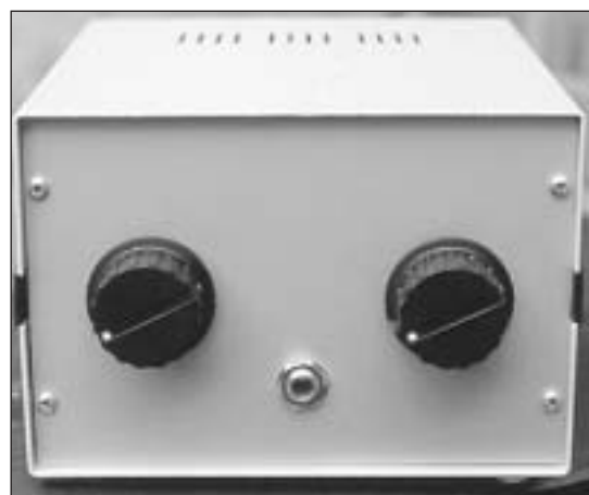
PHOTO 2: The final version of the headphone amplifier in a metal cabinet. I used separate volume controls for each channel rather than a dual Alps pot since I like to make occasional small adjustments of channel balance.
