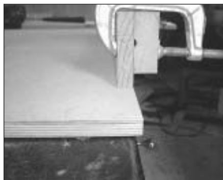
PHOTO 6: Reinforcing the push-bar.
