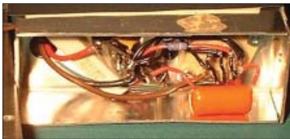
PHOTO 6: The simple oscillator circuitry is mounted under the 6KG6A socket.
