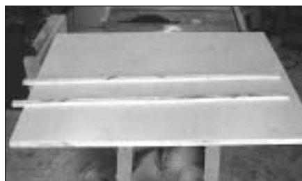
PHOTO 1: One large piece of plywood and two small strips form the basis of the panel-cutting jig.
