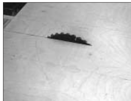
PHOTO 4: Cutting the jig almost, but not quite, in half.
