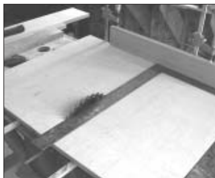
PHOTO 5: Squaring the push-bar to the blade.
