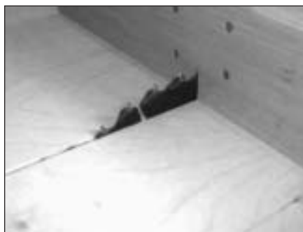
PHOTO 7: The blade passes through the lowermost portion of the push-bar.
