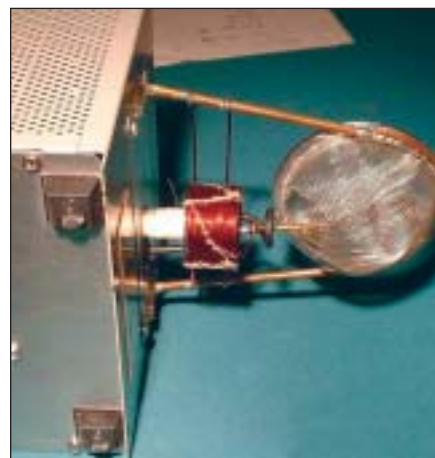
PHOTO 4: Resonant coil, little feedback loop, and Faraday shield.
