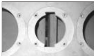
PHOTO 6: Threaded brass inserts were used for mounting the drivers.
