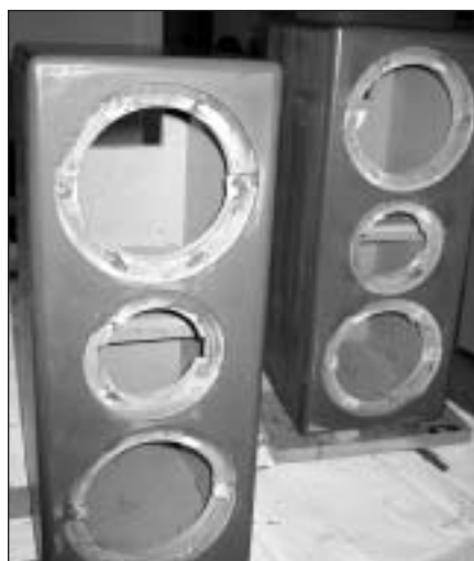
PHOTO 13: Second primer coat is complete, all mounting inserts covered by masking tape.
