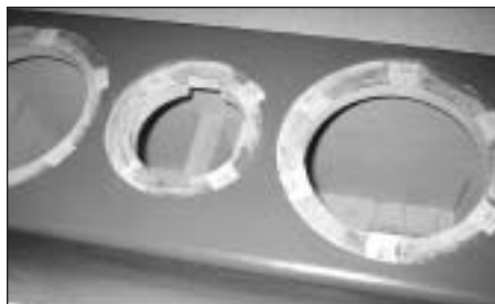
PHOTO 14: Fifth coat of paint completed with the box ready for hardware installation.
