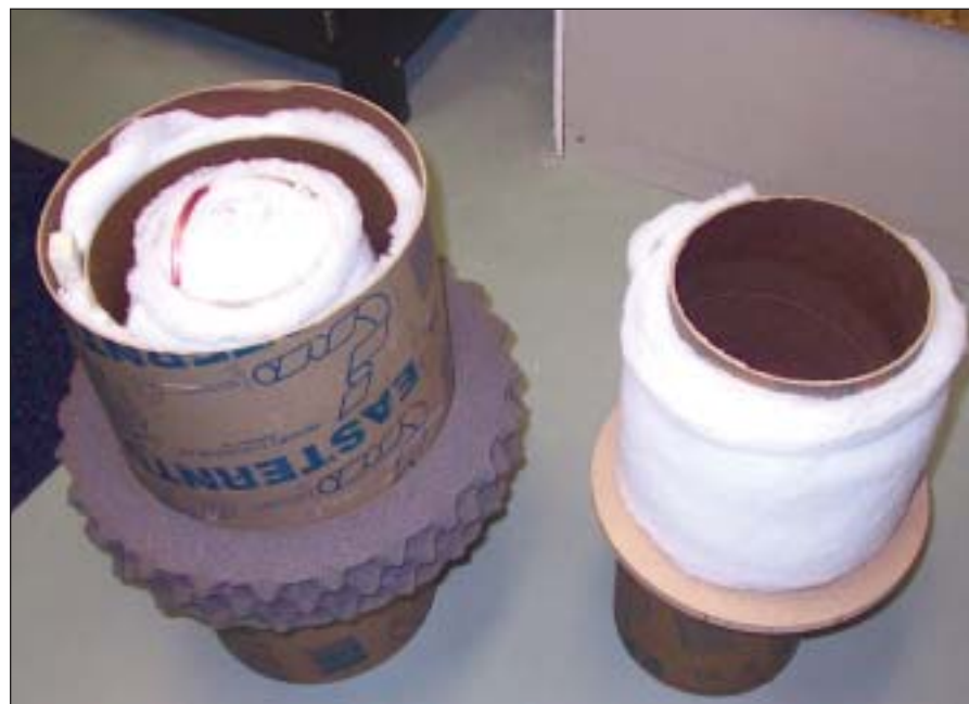
PHOTO 2: Enclosure halves ready for stuffing (one enclosure).
