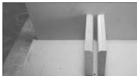
PHOTO 2: The Froy port is unusual located midway between top and bottom of the cabinet. The inner sides of the port walls have been rounded to smooth diffraction in the port. Screws were used to fasten the port walls, and pilot holes are visible for cutting the back opening later with a jig-saw.
