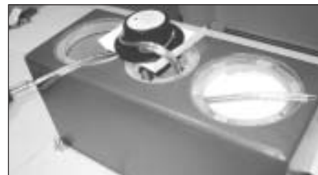
PHOTO 16: Tweeter is connected, stuffing installed and machine screws ready for final mounting of the drivers.
