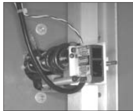
PHOTO 6: The internal laser determines the precise position of the rear of the motor structure.
