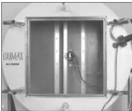
PHOTO 5: A frame inside the test chamber mounts the internal laser.
