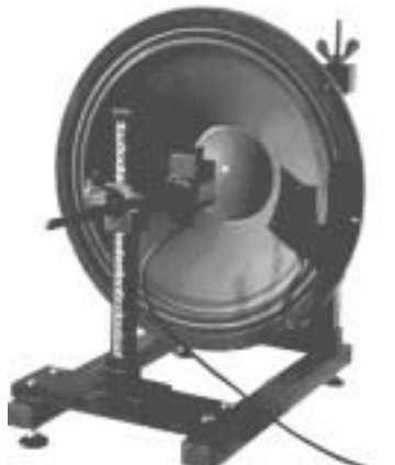
PHOTO 13: A driver mounting stand with laser mount allows diaphragm position information to be collected and sent to the Distortion Analyzer 1.
