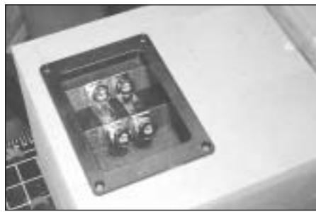
PHOTO 9: The opening for the terminal block is opened after box assembly, and mounting screw locations marked for drilling.
