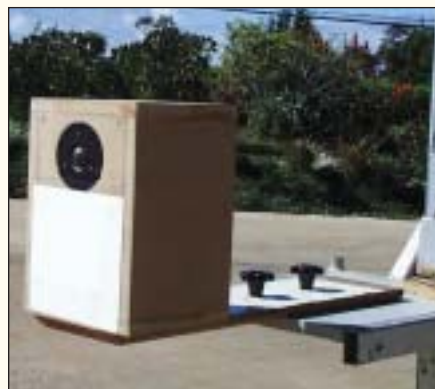
PHOTO 1: Morel MDT-29 tweeter and Vifa P13WH (covered with poster board) mounted in enclosure.
