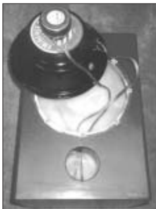
PHOTO 6: Assembled woofer and concentric tweeter just prior to installing the driver assembly.
