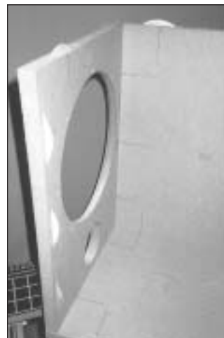
PHOTO 4A: Biscuits in place on inner face of the front panel with mated side and bottom.
