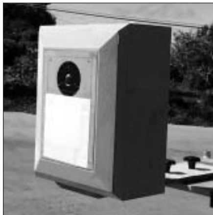
PHOTO 10: Test enclosure with dual bevel, 22°, 45° shell.
