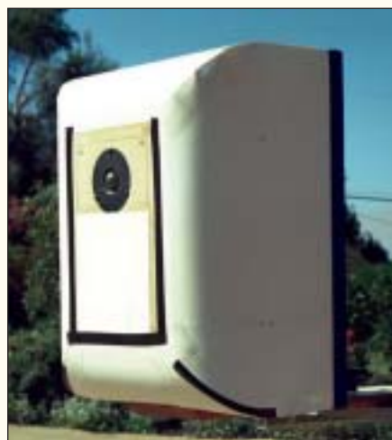
PHOTO 4: Test enclosure with 4" radius shell.
