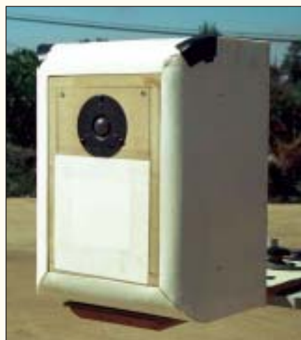
PHOTO 5: Test enclosure with 2" radius shell.
