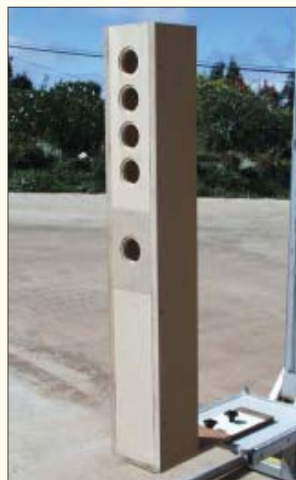
PHOTO 3: A test enclosure that is 8.875” wide and 56” tall.
