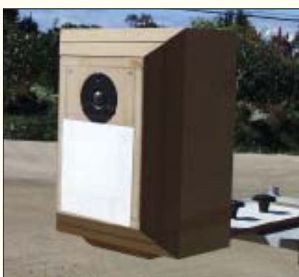
PHOTO 8: Test enclosure with 2", 45° bevel shell.
