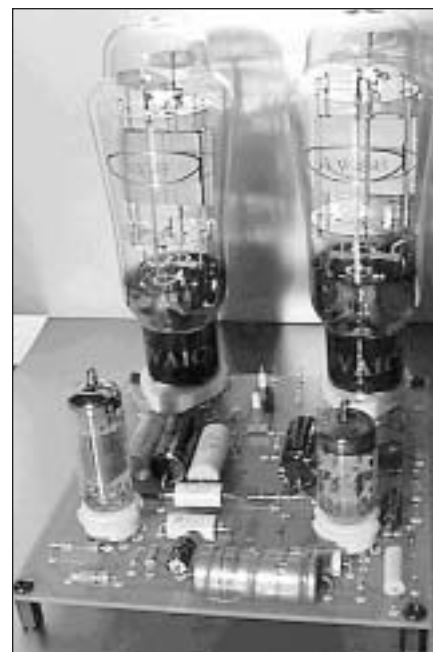
PHOTO 2: Testing THD with VV30 power triodes.
