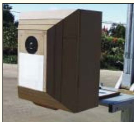
PHOTO 7: Test enclosure with 4", 45° bevel shell.
