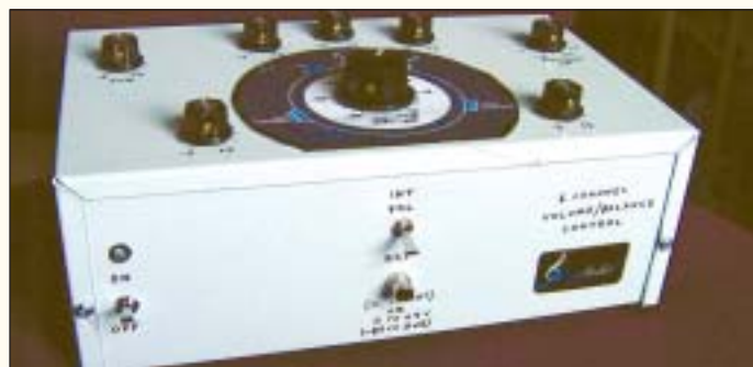
PHOTO 1: The completed 6-channel volume/balance control.
