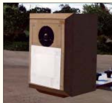
PHOTO 9: Test enclosure with 1", 45° bevel shell.
