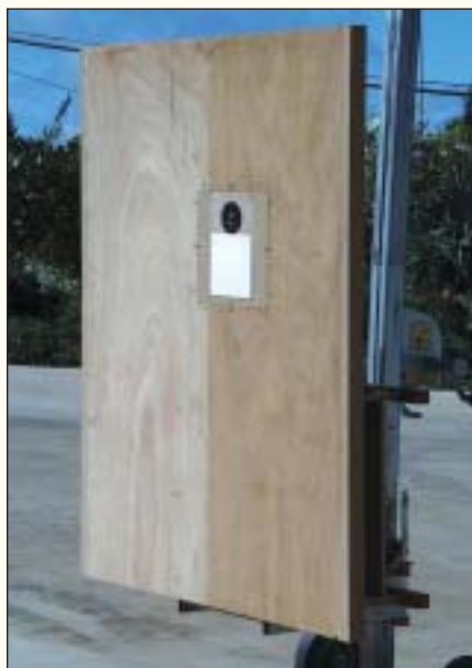
PHOTO 2: Enclosure with drivers mounted on IEC baffle for measurement.
