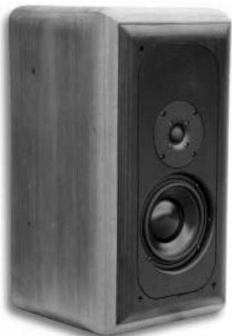
PHOTO 11: Example of grille frame integrated with a stepped front baffle.
