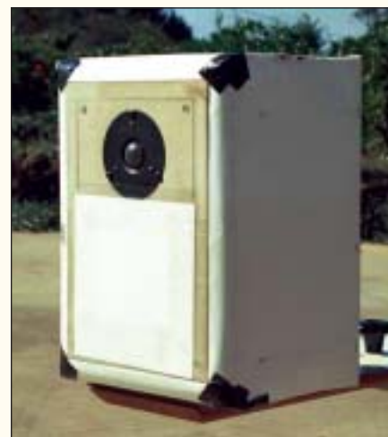
PHOTO 6: Test enclosure with 1" radius shell.
