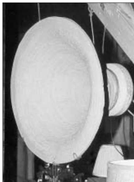
PHOTO 1: The author's axisymmetrical horn design.
