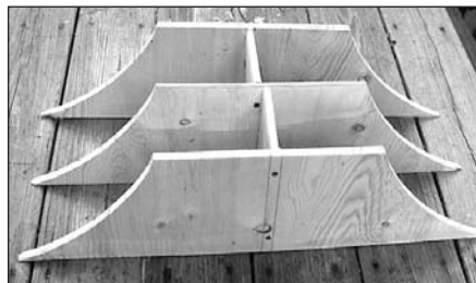
PHOTO 4: The throat horn sides/partition/divider assembly.
