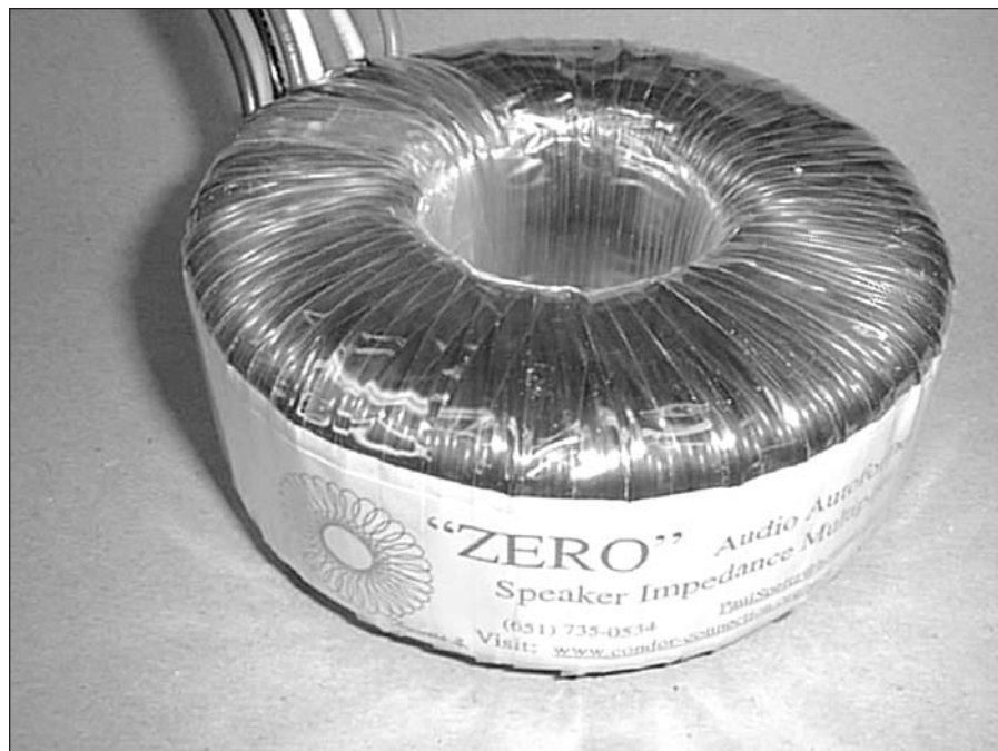
PHOTO 6: The ZERO autoformer. Using its 2:1 winding ratio leads, a 4:1 impedance conversion is achieved.
