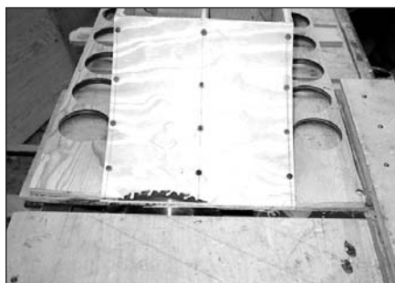
PHOTO 7: Truing the throat horn assembly on panel cutting jig.
