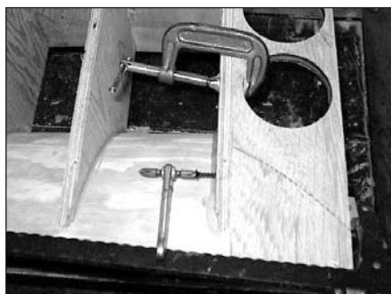
PHOTO 6: Using clamps and right-angle ratchet driver to attach horn support.
