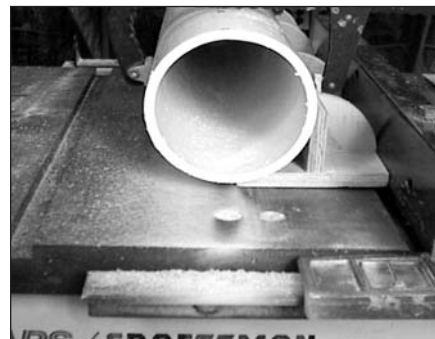
PHOTO 18: Halving PVC is easy with a home-made jig.
