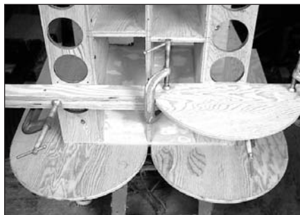
PHOTO 13: Aligning a back support.
