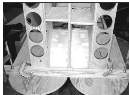
PHOTO 9: Using guide board and clamps to align throat horn on top.
