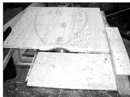
PHOTO 8: Simul-cutting the top and bottom on panel cutting jig.
