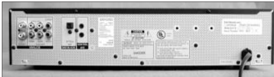
PHOTO 2: Rear view of the SCD-CE775. The stock PC-mount RCA jacks for the two-channel outputs are replaced with Cardas GRFA connectors by SACDmods.
