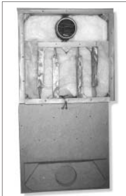
PHOTO 2: Treble speaker assembly with fiberglass installed before attaching back panel.
