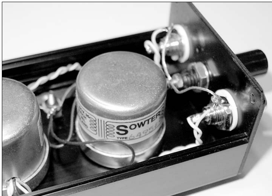
PHOTO 7: Close-up of the input jacks. Note the extra ground wire run to the RCA jacks (see text).
