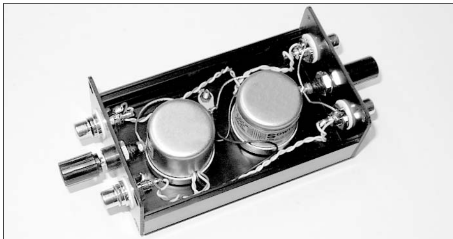
PHOTO 6: The transformers mounted into an aluminum enclosure.
