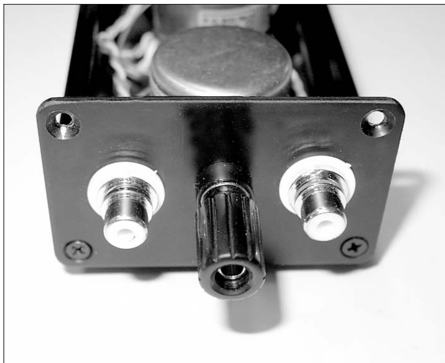
PHOTO 8: The RCA jacks and ground binding posts.
