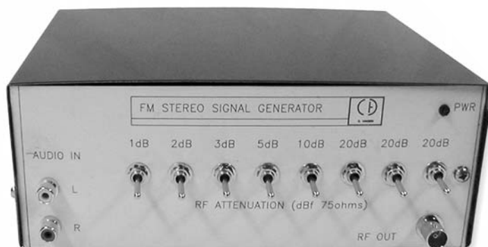
PHOTO 1: Signal generator front view.
