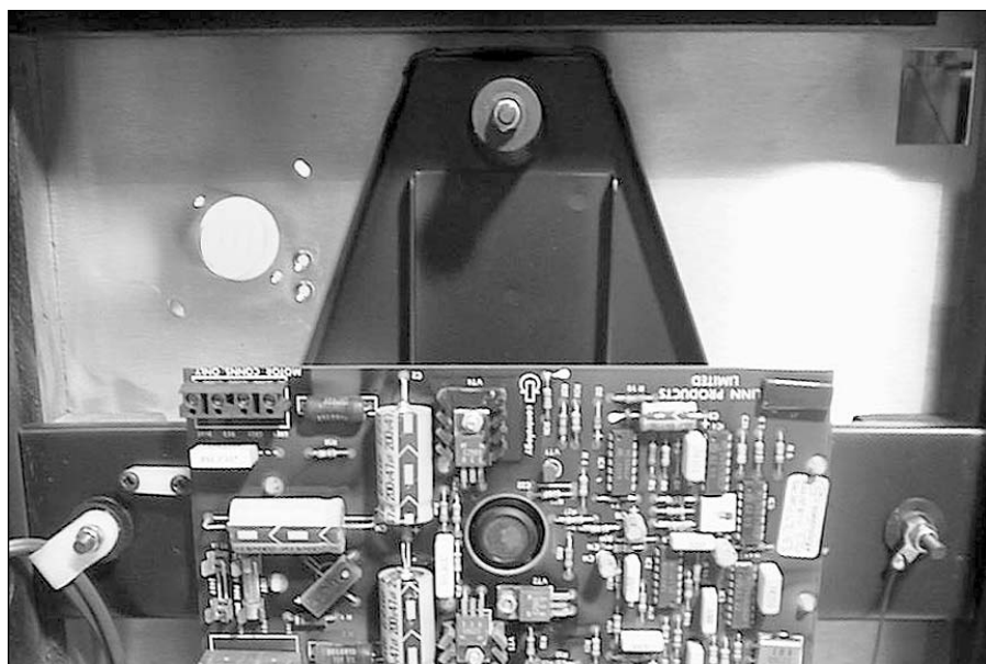
PHOTO 3: The turntable after removal of the Linn motor and power switch.
