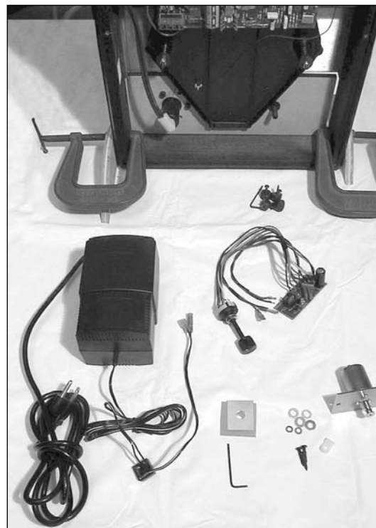
PHOTO 1: The Origin upgrade kit of parts, showing the special optional power supply, which comes with a bridge rectifier with flying leads, presumably to be mounted on the base wall. The turntable is in the background set up for modification, held by C-clamps and plywood scraps.
