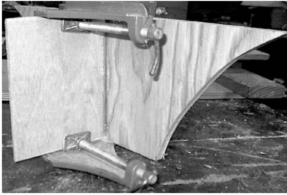
PHOTO 2: The throat-horn divider clamped to throat-horn side.
