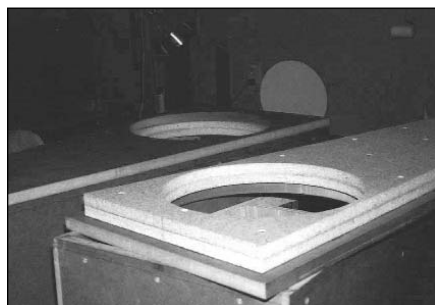
PHOTO 10: View of bass cabinet with woofer cut-out.
