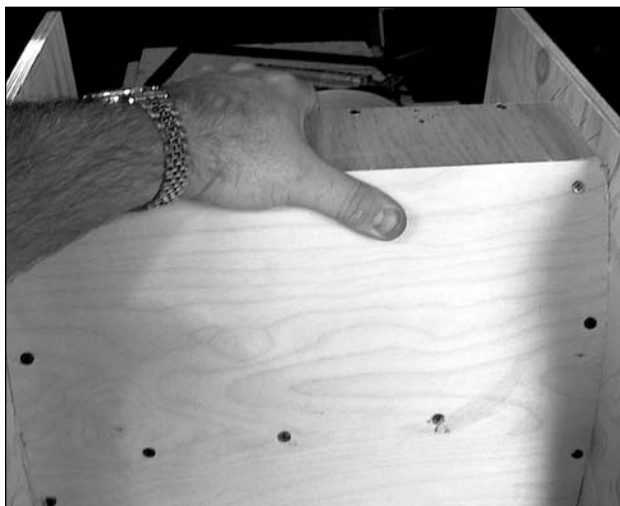
PHOTO 12: Holding the sheathing in place. The \frac{1}{8} " sheathing bends easily, no clamps required.
