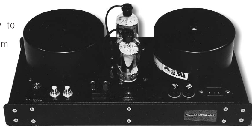
PHOTO 1: Monoblock 100W cascode power amplifier. The chassis is an LMB UPS175-7-14.
