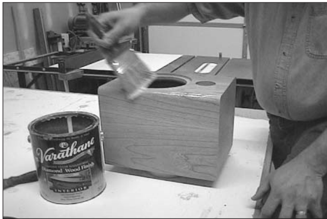
PHOTO 27: Applying urethane finish.
