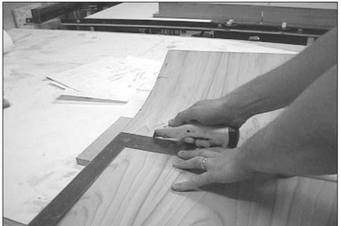
PHOTO 19: Cutting the veneer.
