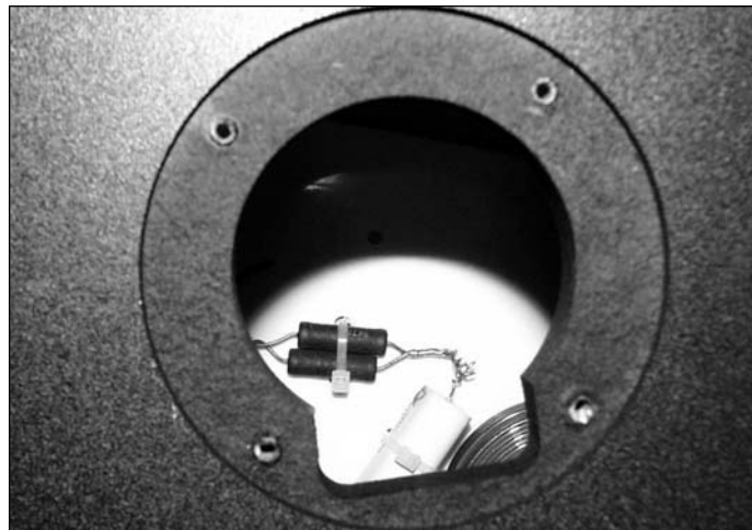
PHOTO 9: Crossover mounting screw visible through tweeter opening.
