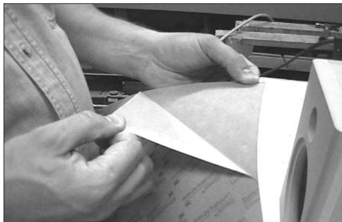
PHOTO 20: Peeling veneer backing.
