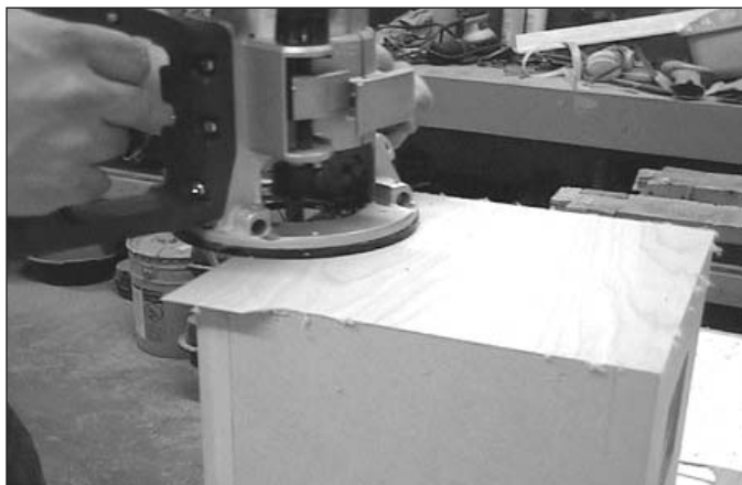
PHOTO 23: Using a laminate trimmer to trim the top veneer.
