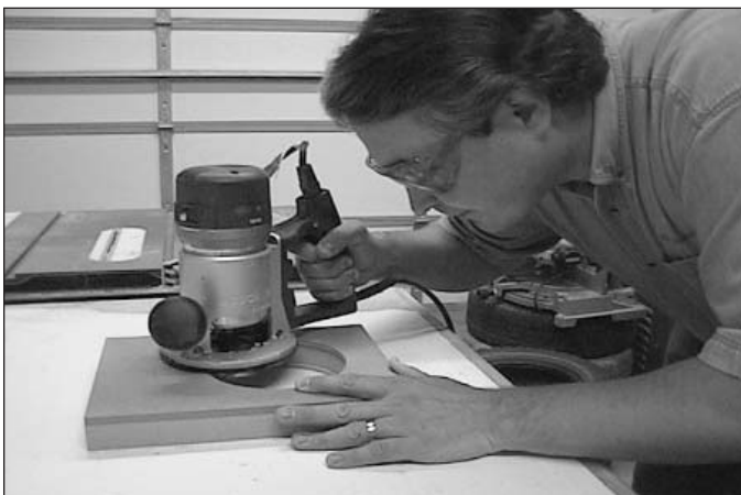
PHOTO 8: Routing a driver hole with a template.
