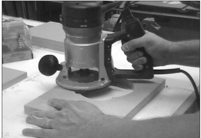
PHOTO 9: Routing the driver recess.
