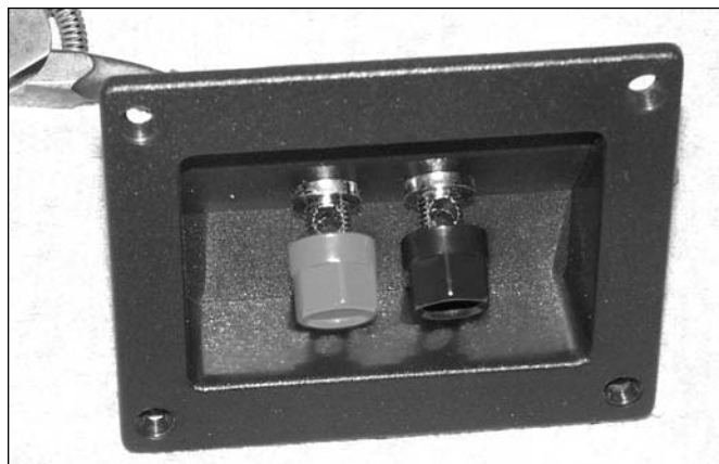
PHOTO 6: Proper alignment of binding posts.
