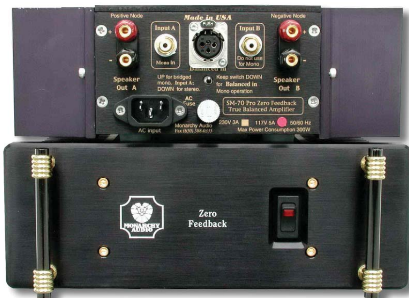
PHOTO 1: The SM-70 Pro power amp, front and rear. Like its predecessor, this stereo power amp performs best when used as a balanced-input monoblock.
