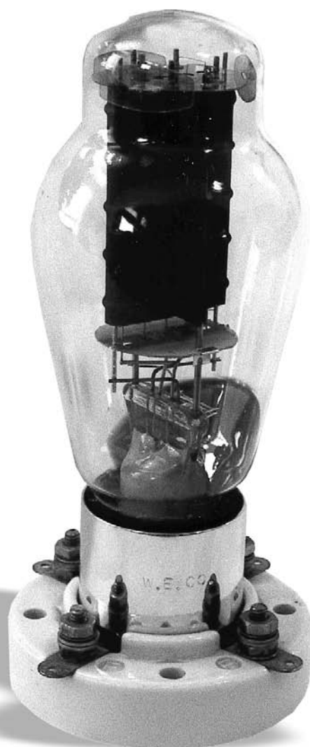
PHOTO 1: WE 300 B-style socket after finishing and plating.
