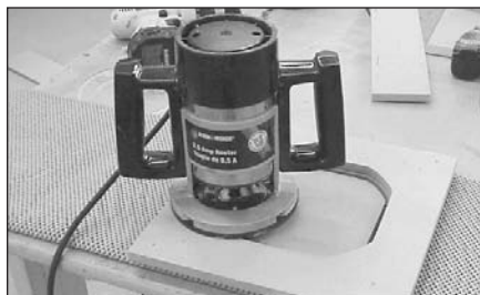
PHOTO 7: After setting router to depth, remove all excess within pattern.
