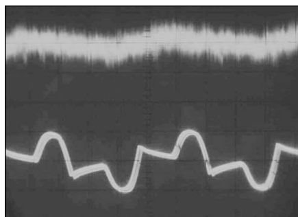
PHOTO 12: Oscilloscope pattern showing output noise (top trace) and the current through the plate winding, using the toroidal transformer. The noise from the transformer stray flux is gone.
