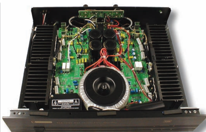
PHOTO 3: HCA-1000A interior view.
