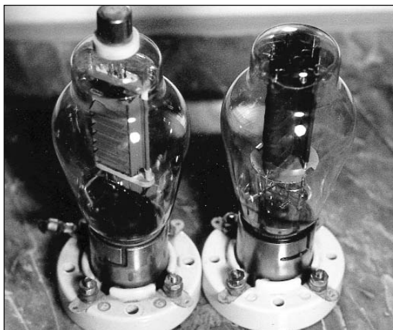
PHOTO 4: Rear view of modified sleeve readily shows difference in pin locations. At left, 812A triode; at right, 300B triode with rotated bayonet pin.
