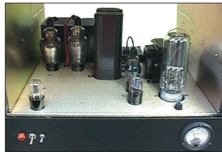
PHOTO 5: Front view of amp showing front-panel controls. Power indicator, far left. Switch next to power indicator is the main power switch. Far-right switch is the 211 filament "operate/standby" switch. Right-hand side of panel, contains an optional current meter to monitor 211 output tube current.
