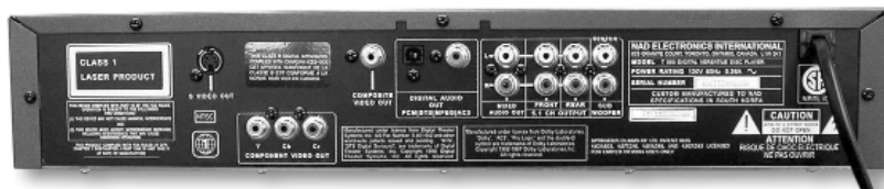
PHOTO 2: Rear panel of the T550. The player has built-in Dolby 5.1 decoding and the six required outputs. Separate stereo/mixdown outputs are provided for two-channel operation. Component, composite, and S-Video outputs are also included.
