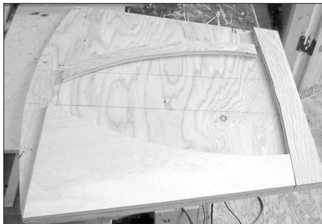
PHOTO 7: Checking brace patterns against cabinet top.
