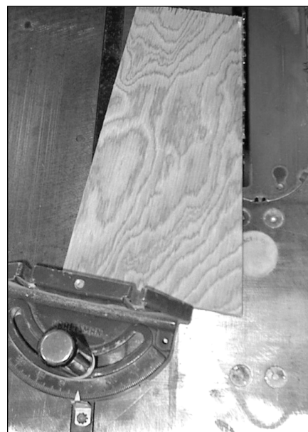
PHOTO 5: Cutting angled piece of plywood to modify panel cutting jig.
