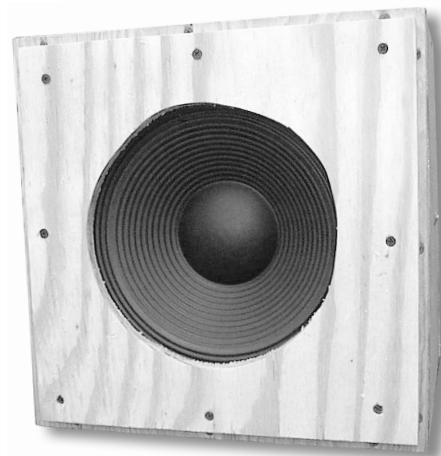
PHOTO 1: Test box w/10" driver.
