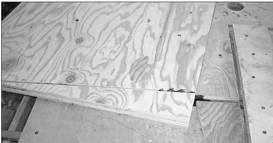
PHOTO 6: Cutting cabinet top using modified panel cutting jig.
