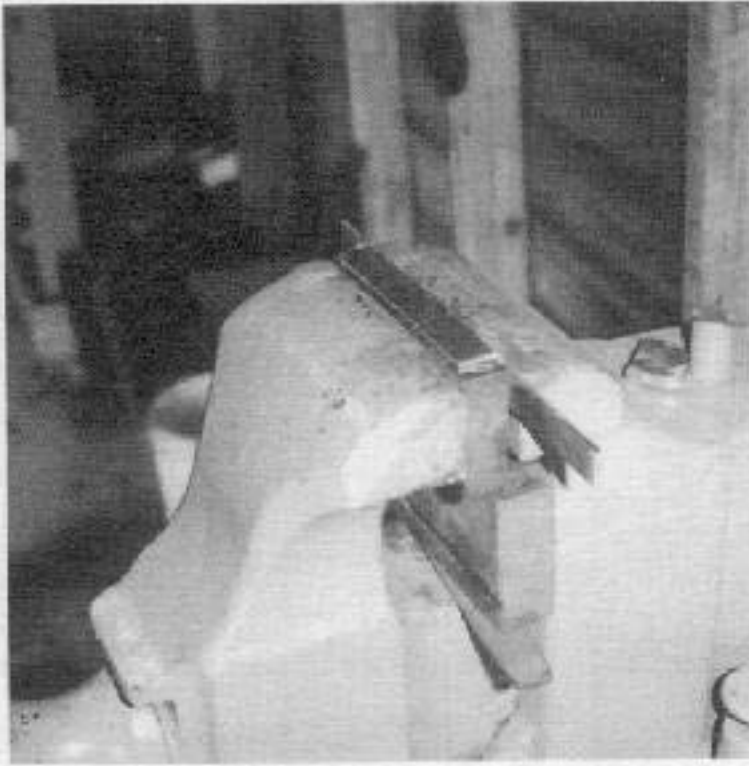
Sides are formed with block and hammer.
