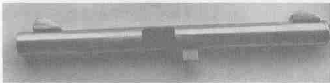
Blocks for mounting brackets are welded on lower side.
