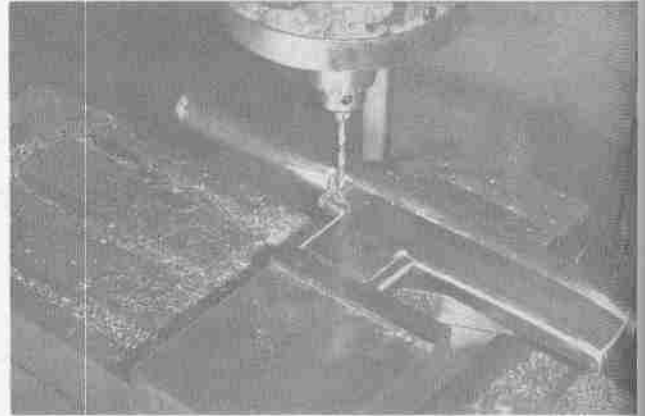
The front screw hole is drilled simultaneously through the upper and lower receivers while they are clamped together.
