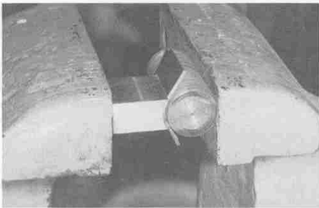
Vise jaws are drawn together, forming curve on bottom.
