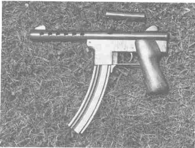
The open-bolt assembly shown just above the gun is interchangeable with the closed bolt.
