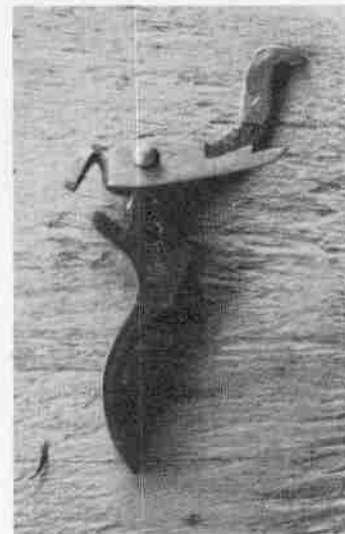
Trigger with trigger bar pinned in place.
