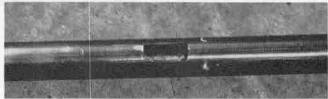
Holes are welded, fusing bushing to receiver body. If welds are built up above the surface and dressed back flush, no evidence of welding will be seen.
