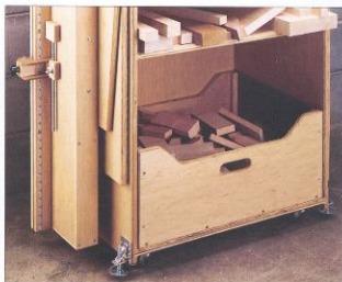
The removable scrap bin is big enough to hold lots of cut-offs. But the handles make it easy to lift out and empty.
