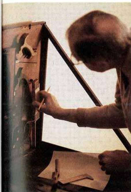
Lynch prefers a folding carpenter's rule, left, because it won't snap back as a steel tape might. Holding his bevel gauge handle parallel to the chest corner, he angles its tongue to match the dovetails, above. He records the angle with a protractor. For something as irregular as this tavern table leg, he uses a simple pen holder to trace contours. The Plexiglas edge of the wooden upright is set directly over the angled pen. As you run the plastic along the piece, the pen records the contour on paper on the instrument's base.
