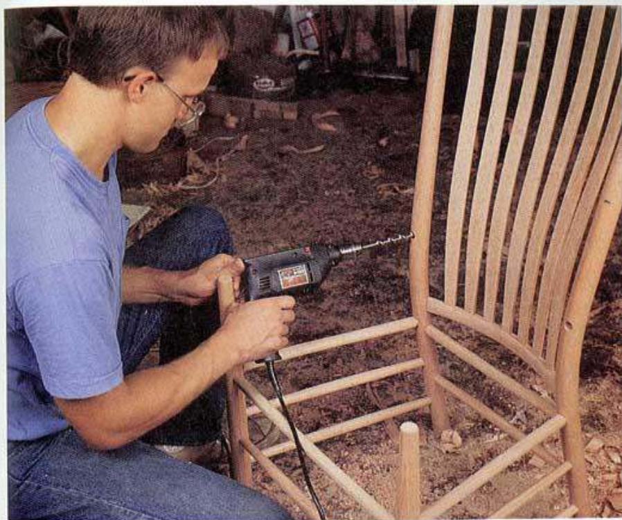
Above: Boggs' bent-back rocker design evolved as he experimented with changes in early chair models. Left: With a Forstner bit in a power drill, the author bores the armrest mortise in the rear leg post. The front leg post serves as a guide as he eyeballs the mortise position.
