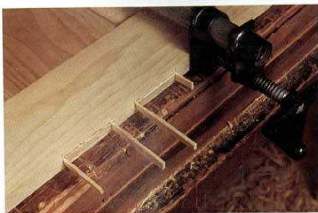
Above, wedges and pins lock the tenons securely without glue. The wedges are driven in above and below the tenons until they seat firmly. Below, pins made from rounded square stock are driven into \frac{1}{4} -in. through-bored holes.
