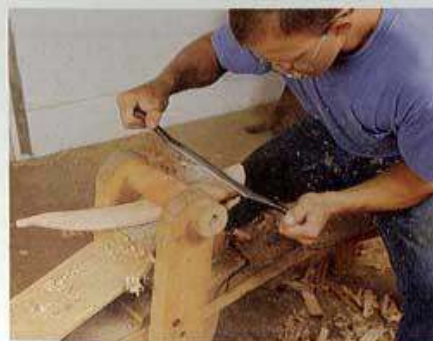
The author is shown working at a shaving horse, rough-shaping a green-wood armrest. The job goes quickly because green wood is easy to carve. Boggs removes wood efficiently with a drawknife.
