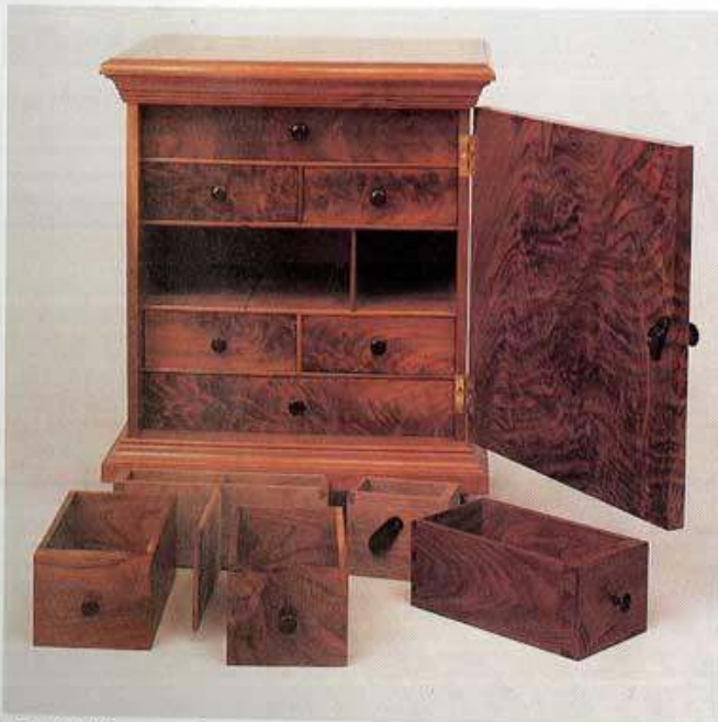
This William-and-Mary spice box has more drawers than first meet the eye: Two are concealed behind shallow conventional drawers, with one, the dual drawer, attached to a sliding partition. A third secret compartment located behind the cornice molding can be accessed only by moving the back panel.
