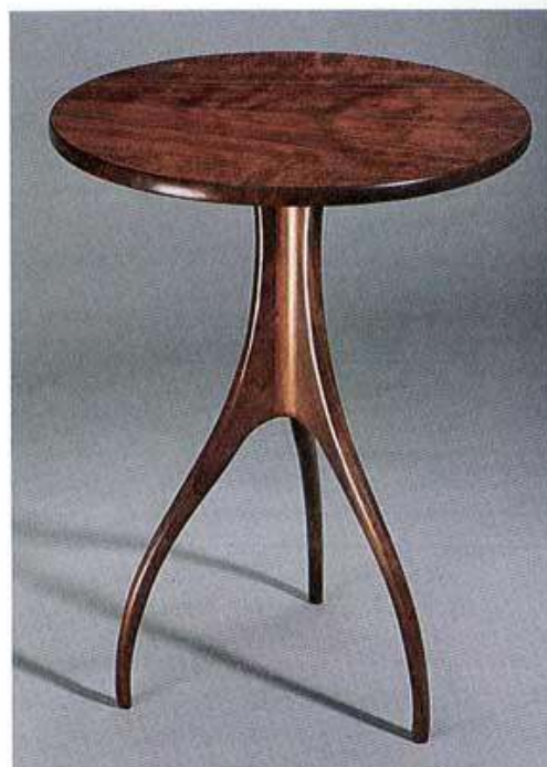
The pedestal of this sleek update of the Shaker classic is constructed by laminating filler blocks in the gaps between the legs and shaping the juncture with a round-bottom plane. This table is made of mahogany and finished with French polish.
