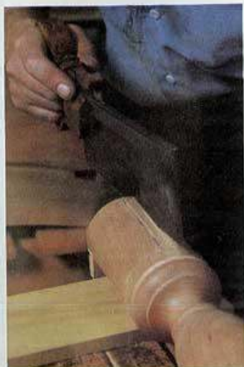
Use a backsaw to cut just inside the layout lines of the dovetail housing, left, then pare to the lines with a sharp chisel. The waste will come out in long strips. Once the leg goes in an inch or so, use the first part of the joint to guide the chisel to the full length of the housing, right.
