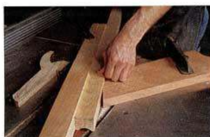
To cut a cove molding, run the workpiece along a fence angled to the blade. Make several shallow cuts, then rip the workpiece in half. Hold the work against the fence with a featherboard, using a push stick to finish the cut.
