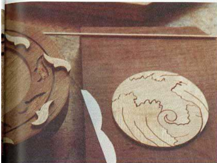
The cherry block is grooved and excavated, left, for the inlay. With the block attached to a faceplate, above, a shoulder is cut on the face to the final diameter of the pattern before a thin disc is cut off. The text below describes a safe tablesaw method, in which the block is left square, not turned round.
