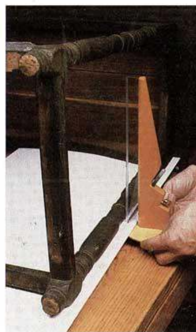
Lynch prefers a folding carpenter's rule, left, because it won't snap back as a steel tape might. Holding his bevel gauge handle parallel to the chest corner, he angles its tongue to match the dovetails, above. He records the angle with a protractor. For something as irregular as this tavern table leg, he uses a simple pen holder to trace contours. The Plexiglas edge of the wooden upright is set directly over the angled pen. As you run the plastic along the piece, the pen records the contour on paper on the instrument's base.
