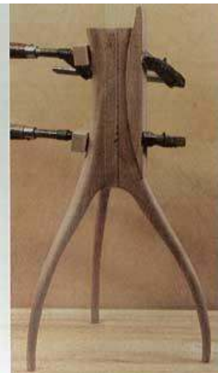
These three photos show the fixture and clamping arrangements used for assembling two legs with a filler block (left); two filler blocks with a leg (center); and the final pedestal glue-up (right). A scrap piece, left over from the bandsawing of the legs, is used as a caul.
