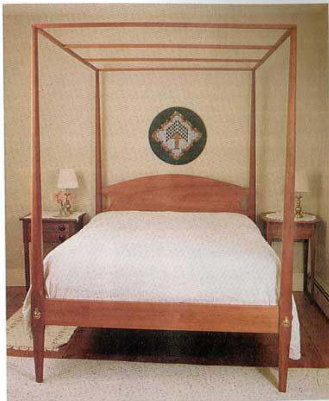
A pencil-post bed with traditional tester or canopy frame is shown above. The eight-sided, tapered posts are mortised to receive the four bed rails, which are held in place with bed bolts concealed behind the brass bolt covers. There are no glued joints, so the entire bed can be disassembled for ease of transport.
