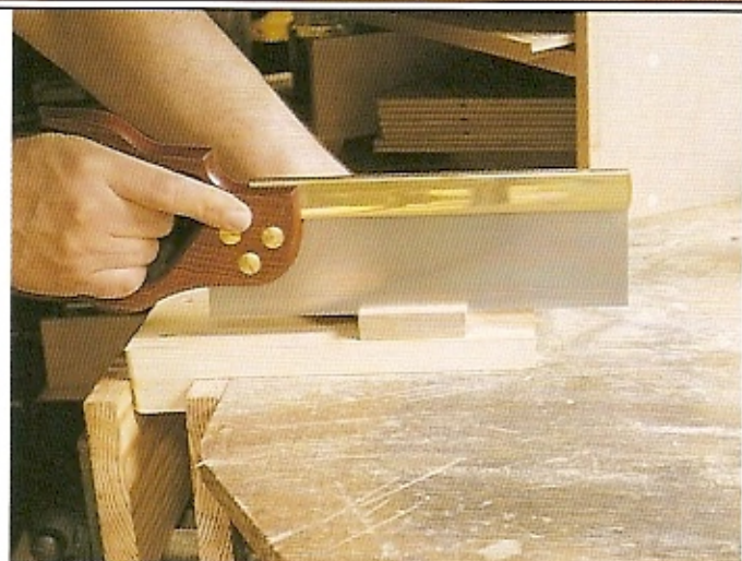
11 Cut the drawer faces to rough length.
