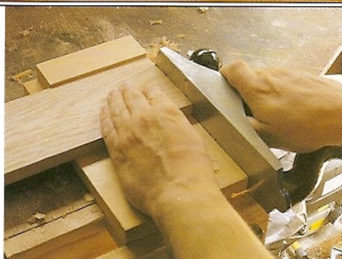
12 Final fit the drawer fronts using your handplane.
