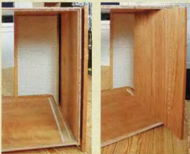
SEE HOW THEY RUN. With the back of the cabinet removed (far left), the two tambours can be fed in from the right rear side and slid around to their respective positions. Then the two partition panels are fitted so that the tambours are concealed when the doors slide into the case (left).
