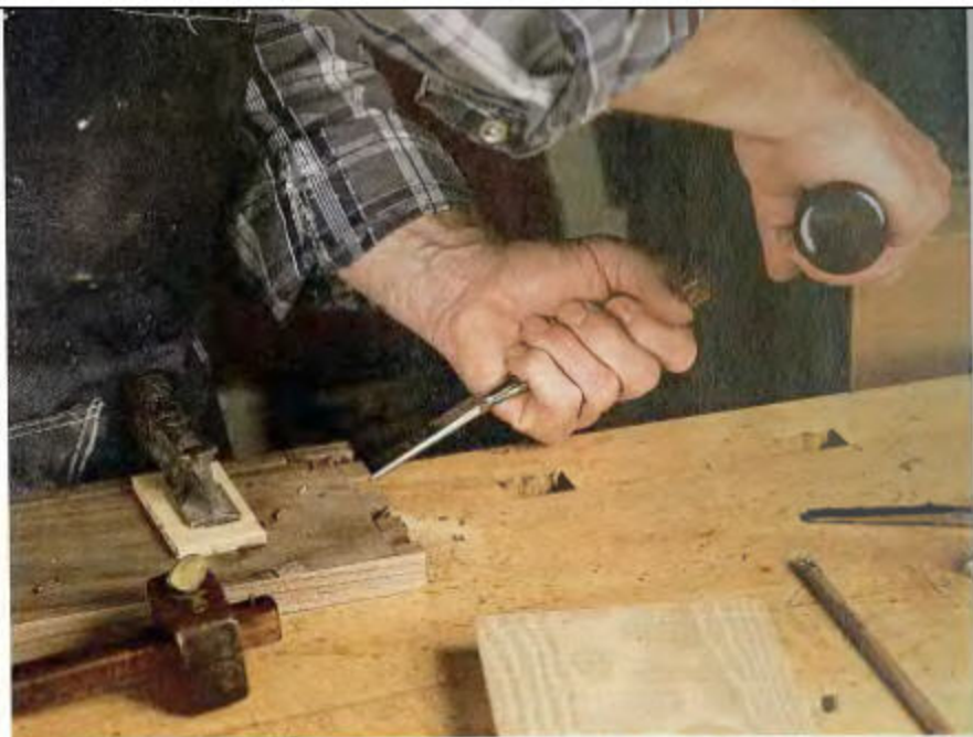
5. POSITION YOUR CHISEL 45° AWAY FROM YOUR BODY, about halfway between baseline and the end of the board, bevel up. Whack the chisel with a mallet, gradually moving the chisel back to the end of the board, working down through the waste between the pins.
