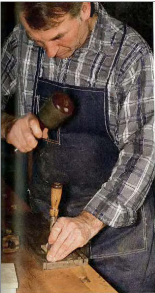
4. CHISEL BASELINE. Position a paring chisel just ahead of the baseline, bevel out. Tap the chisel with the mallet. The bevel drives the chisel to the scored line, preventing tearout.
