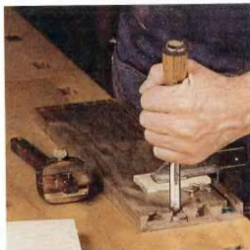
6. ALTERNATE CHISELING FROM THE END with perpendicular blows at the baseline that free the waste.
