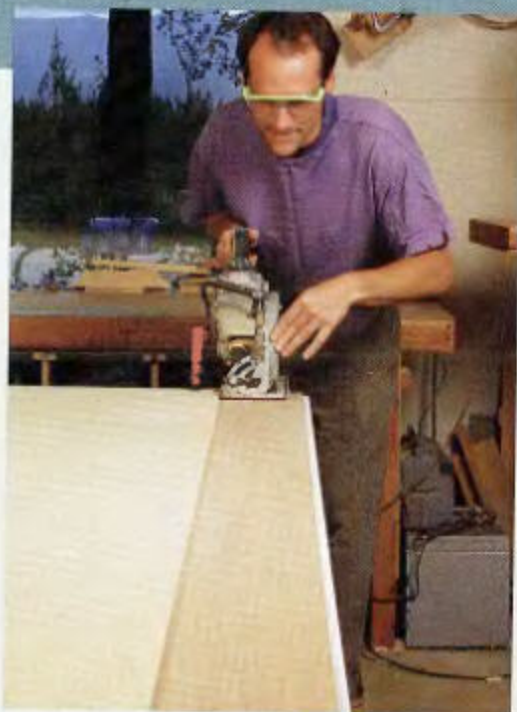
CUTTING A PLYWOOD SHEET. A second sheet of plywood makes a serviceable edge guide for rough-cutting large sheets.
