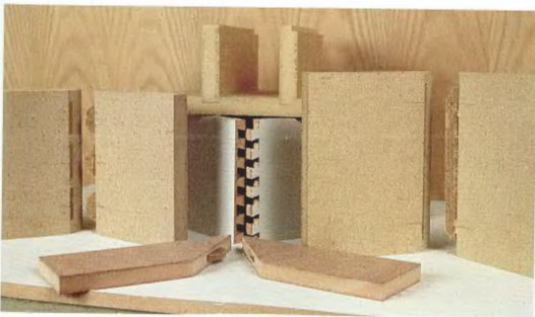
A WIDE VARIETY OF JOINERY is possible with MDF. Examples shown here surrounding a routed dovetail joint are, clockwise from left, biscuits, dado, rabbet and dado, spline miter, and biscuited miter. The background is a sheet of factory-veneered MDF.
