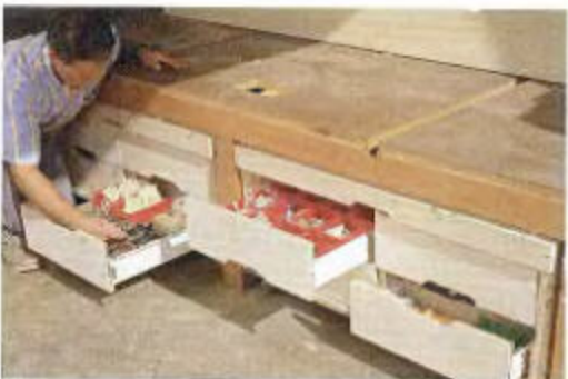
DRAWERS MAKE USE OF FLOOR SPACE. A two-part assembly table rolls under the platform when not in use. Aligned by biscuits and clamped together, the table has slide-out bins in back.
