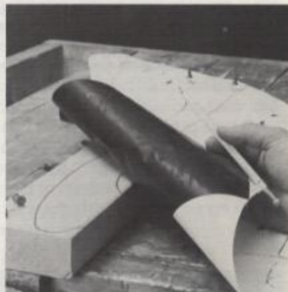
1/Once you've made a full size drawing of the Side View, you can use carbon paper to transfer the shapes of the parts to the wood.
