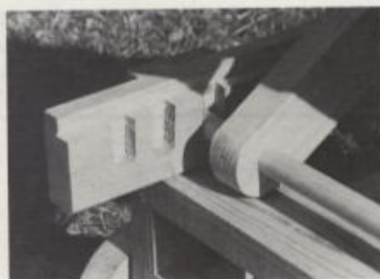
3/ The four notches in the ends of the sides allow you to adjust the back to four different positions. (One notch is hidden behind the brace.)
