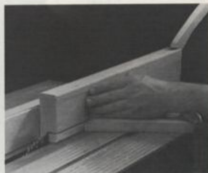
2/ Then cut the width of the rabbets. On the second cut, be careful not to leave the waste in between the saw blade and the rip fence. If you do, it will kick back.
