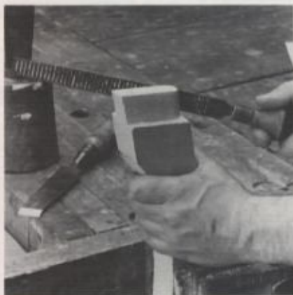
5/Round the tenons with a chisel and a rasp to fit the mortises.
