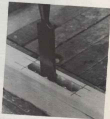
4 To make a mortise, first drill a series of holes. Then clean up the long edges of the mortise with a chisel.
