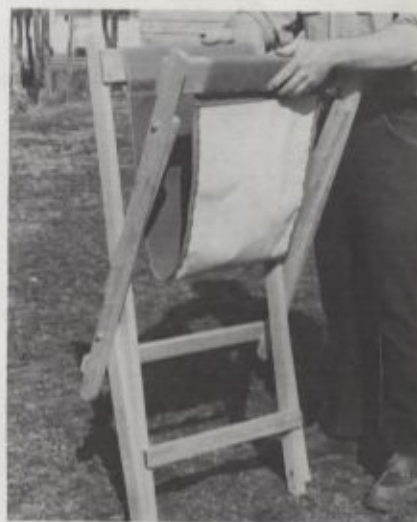
3/ To fold up the chair frame, pick it up by the hangers and bring the hangers together.
