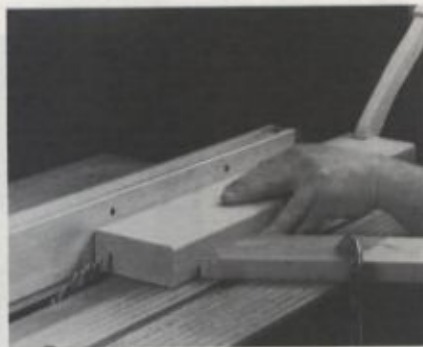
1/ Make the rabbets in the rails in two cuts. First, cut the depth of the rabbets...
