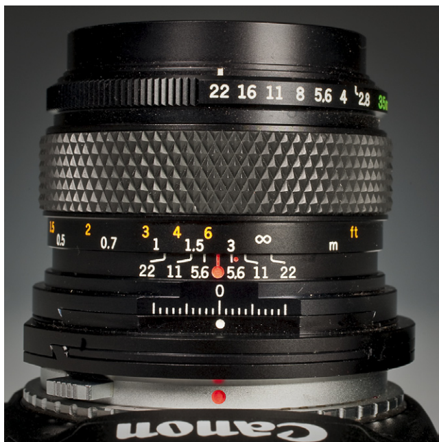
Manual focus lens showing DOF scale and lens focused to HFD
