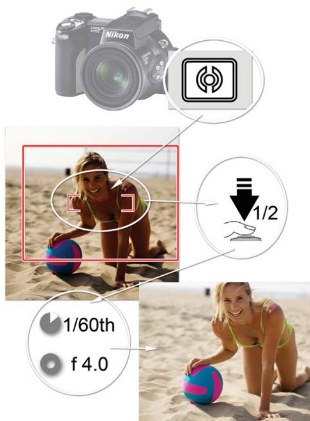
Figure 14.10 By pressing down the shutter button halfway it is possible, with many cameras, to lock the exposure settings used to capture a scene. As the metering system will try to average the scene's tones to match a mid-gray, photographers should carefully choose the parts of the picture that they use as exposure references. Pick a subject that is too dark and the picture will be overexposed. Use a section of the scene that is too light and the image will be underexposed.
