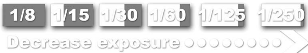
Figure 8.3 The shutter speed controls both the amount of light entering the camera and the way that action or movement is captured. Fast shutter speeds freeze the action, whereas slower settings blur the movement.
